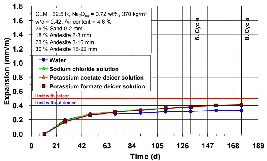
Figure 5: Expansion during the cyclic climate storage for a tested pavement concrete with potentially reactive andesite
