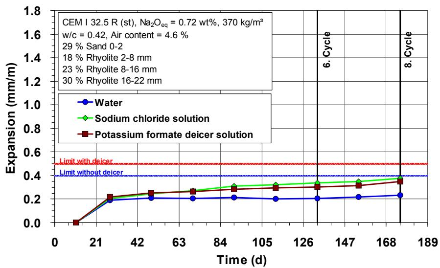
Figure 6: Expansion during the cyclic climate storage for a tested pavement concrete with potentially reactive rhyolite
