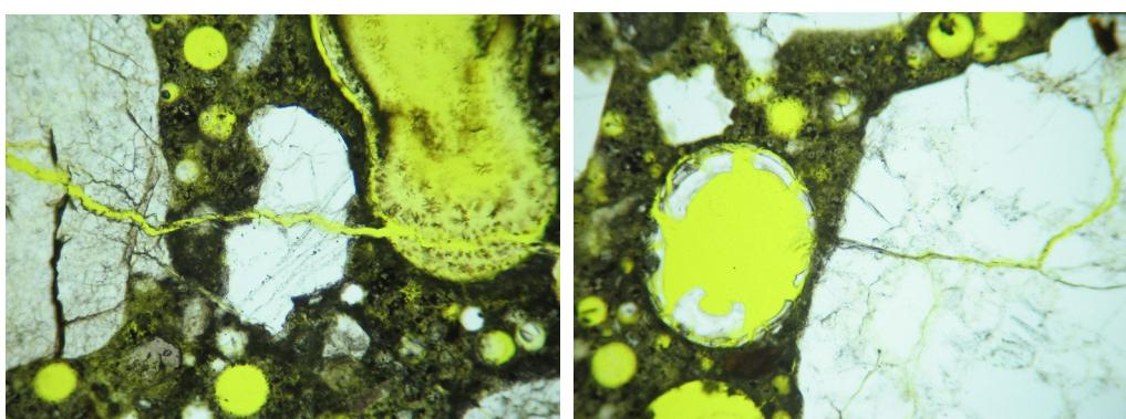
Figure 10: Thin section images after 8 cycles of performance-testing, cracks in granodiorite grains and ASR-gel in air voids
