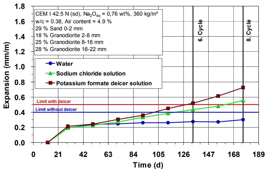
Figure 7: Expansion during the cyclic climate storage for a tested pavement concrete with potentially reactive granodiorite
