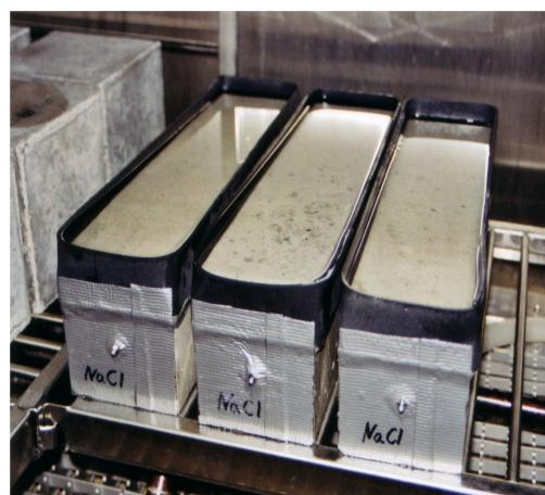
Figure 3: Concrete prisms with foamed rubber tape and applied deicing solution at the upper surface in the special climate simulation chamber
