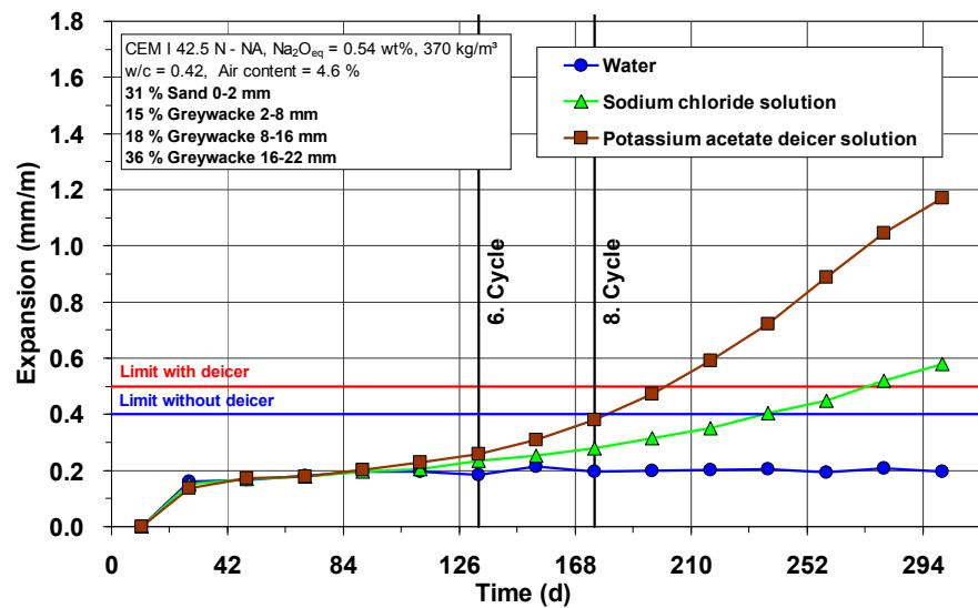
Figure 11: Expansion during the cyclic climate storage for a tested pavement concrete with reactive greywacke and low-alkali cement
