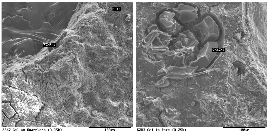
Figure 9: ESEM/REM images of ASR-gel in tested pavement concrete samples with deicer solution
