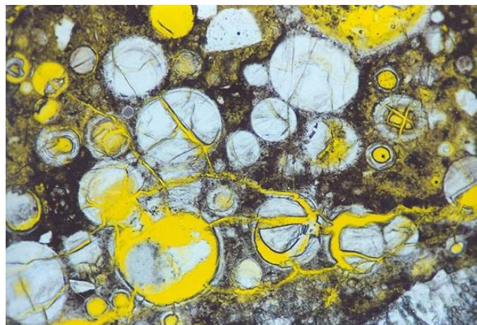
Figure 8: Thin section image, ASR-gel in artificial air voids
