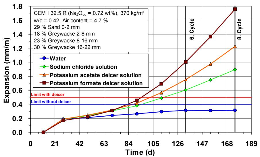
Figure 4: Expansion during the cyclic climate storage for a tested pavement concrete with reactive greywacke
