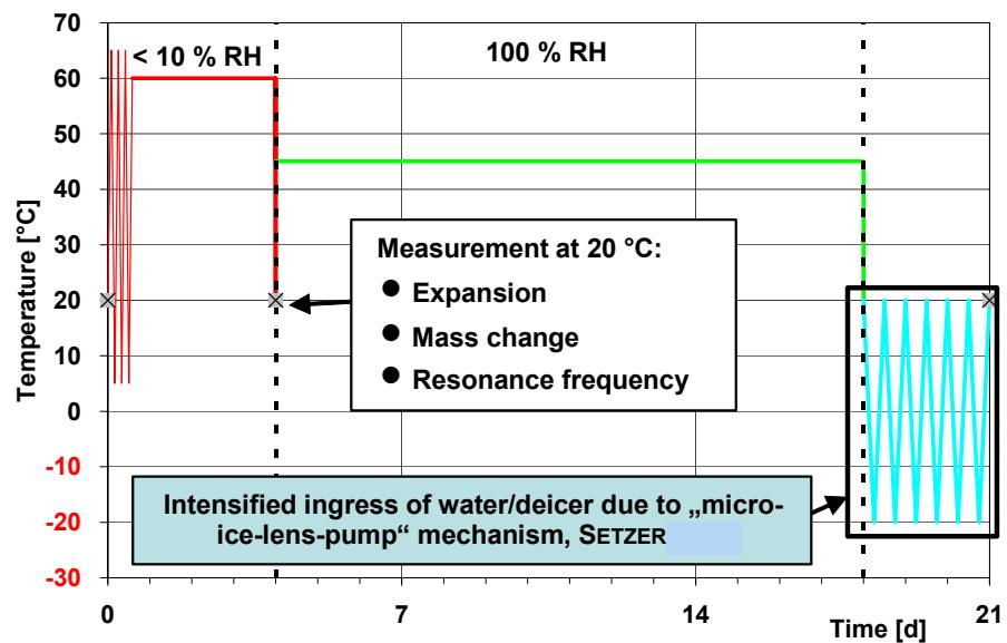
Figure 1: Scheme of cyclic climate storage (one cycle)
