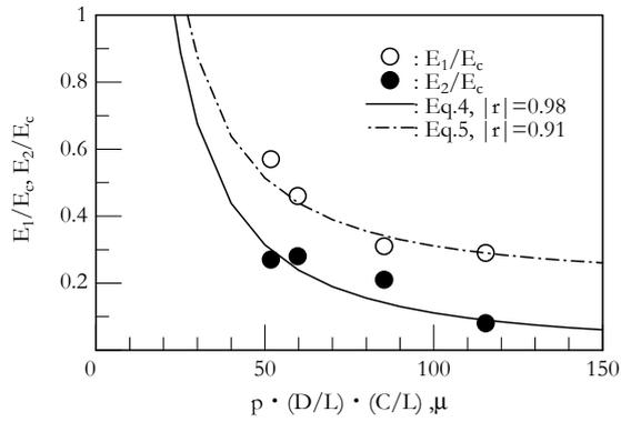
Figure 11: Relationship between Young's modulus of damaged concrete and the coefficient  $\alpha$ .
