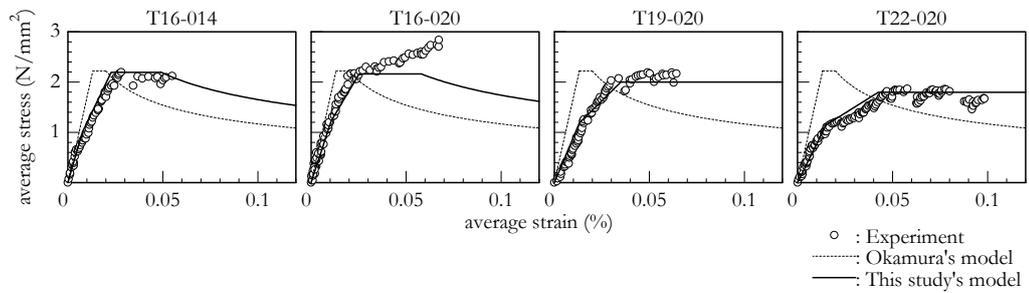
Figure 13: Calculated average concrete stress and strain relationship with factors obtained from parametric analysis.
