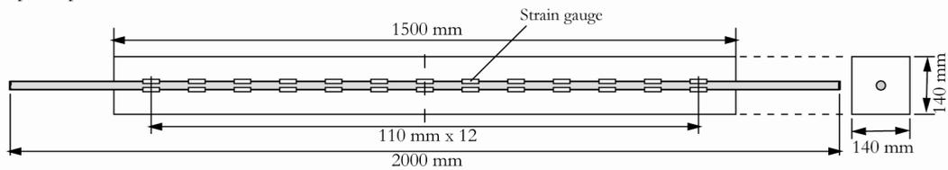
Measurement location of concrete surface strain
