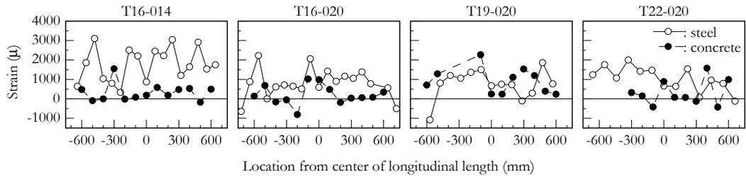
Figure 4: AAR strain distribution of reinforcing bar and concrete surface in the longitudinal direction.
