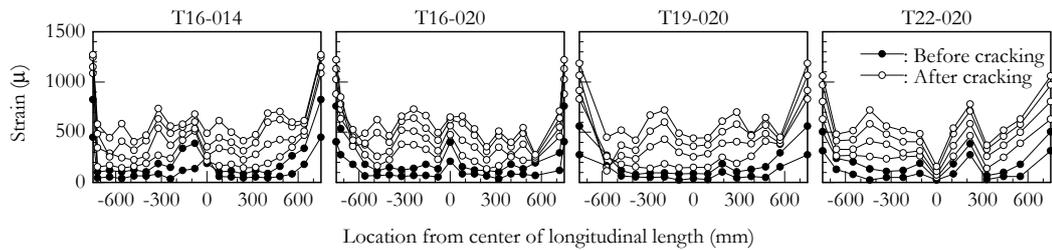
Figure 5: Strain distribution on reinforcing bar under tensile loading.
