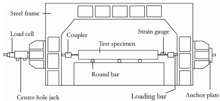
Figure 2: Test setup.
