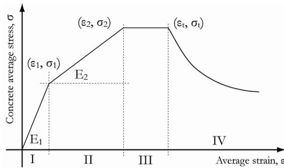
Figure 8: Average stress - strain model of concrete subjected to AAR.
