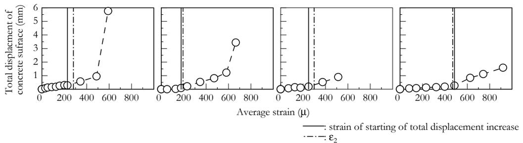
Figure 9: Total displacement of concrete surface - average strain relationship.
