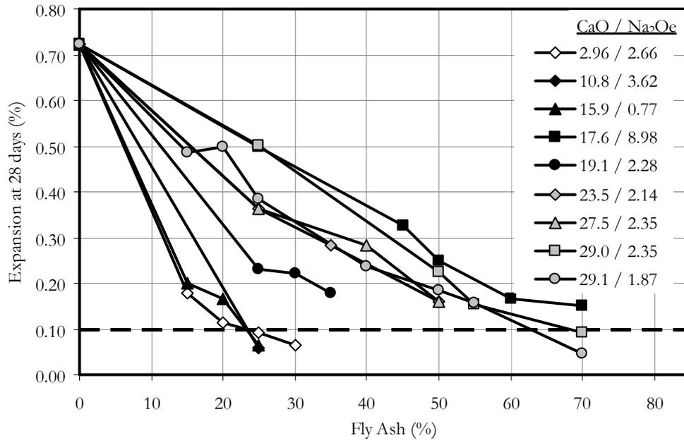
Figure 4: Results of Accelerated Mortar Bar Test for Springhill Aggregate with Various Fly Ashes: 28-Day Expansion.
