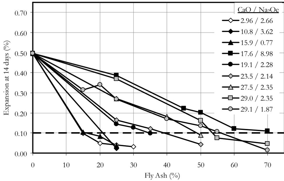
Figure 3: Results of the Accelerated Mortar Bar Test for Springhill Aggregate with Various Fly Ashes: 14-Day Expansion.
