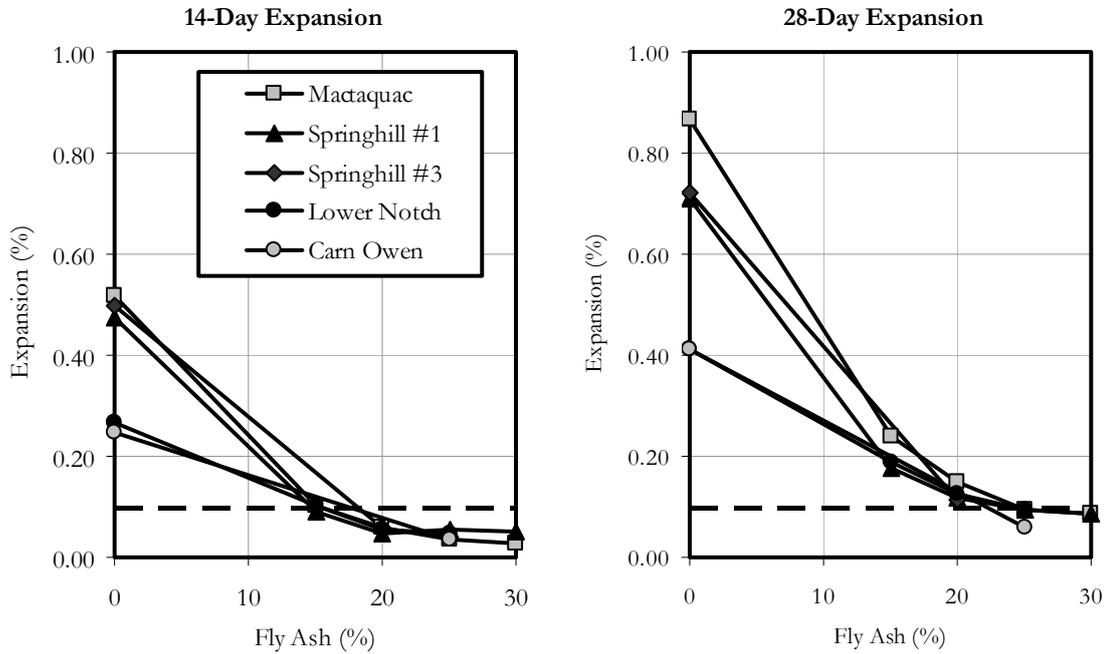
Figure 1: Results of the Accelerated Mortar Bar Test for Belledune (Type F) Fly Ash.
