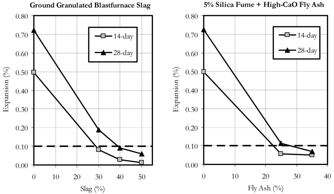
Figure 6: Results of Accelerated Mortar Bar Tests for Springhill Aggregate with Slag (left) and Ternary Blends of Silica Fume plus High-Calcium (29.1% CaO) Fly Ash (right).
