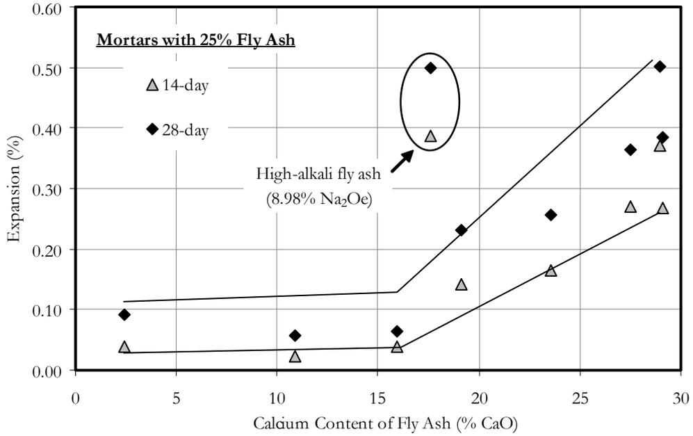
Figure 5: Effect of Calcium (and Alkali) Content of Fly Ashes on Expansion of Mortar Bars Containing Springhill Aggregate and 25% Fly Ash.
