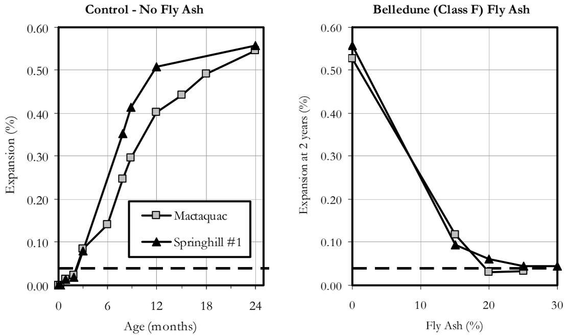
Figure 2: Results of the Concrete Prism Test for Belledune (Type F) Fly Ash.
