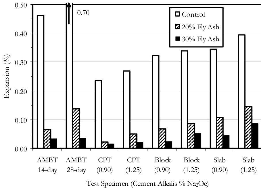
Figure 7: CANMET Expansion Data for Springhill Aggregate with Low-CaO (2.06% CaO) Fly Ash Tested in the Accelerated Mortar Bar Test, the Concrete Prism Test and Outdoor Exposure Blocks.
