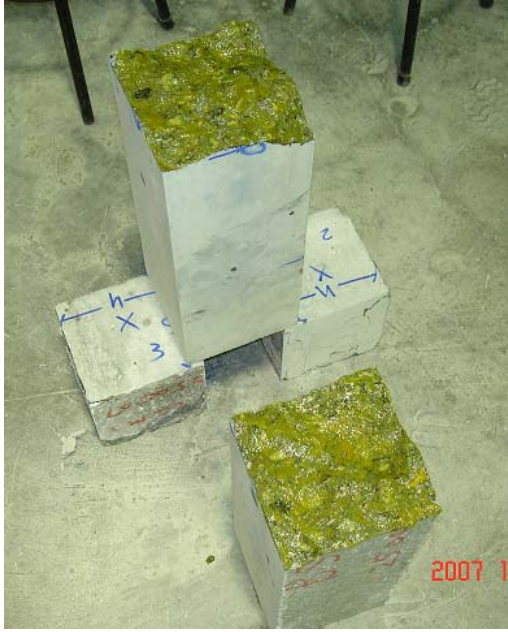
Figure 3: Grease applied on the broken surfaces.
