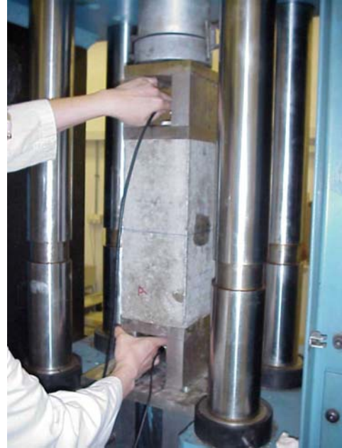
Figure 4: Ultrasonic pulse velocity measurement.
