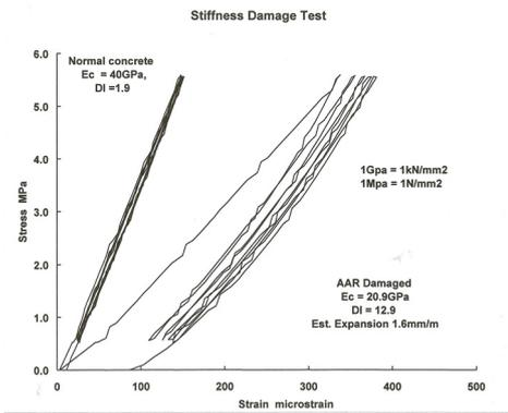
Figure 2. SDT cyclical loading to 5.5MPa on normal and AAR damaged concrete cores.
