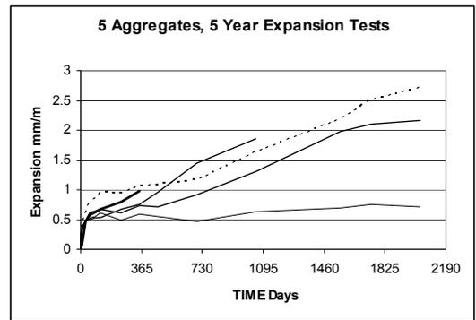
Figure 4a. Long term 20°C Water supply expansion tests. Typical trends for 5 distinct aggregates.
