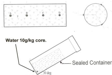
Figure 5, Water supply expansion test to relate expansion to measured water uptake without alkali leaching. Typically uses a 250 long 70mm diameter core with 3 lines of three 50mm Demec gauge lengths to measure the variability of expansions.
