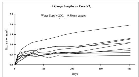
Figure 4b. Long term 20°C Water supply expansion tests. Variability of expansion on Nine 50mm gauge lengths on one core.
