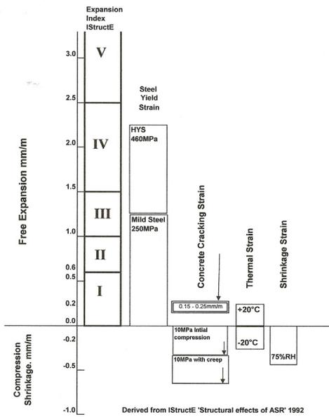
Figure 1 The relative magnitude of thermal and shrinkage strains compared to the IStructE AAR expansion classes
