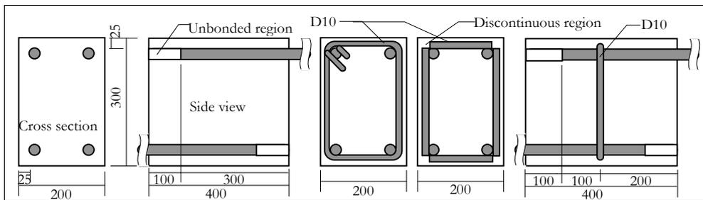
Figure 1: Shape and dimensions of D19 pull-out specimen (dimensions in mm).
