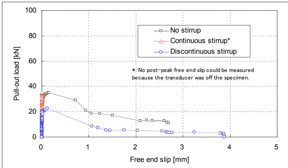
Figure 7: Relationship between pull-out load and the free end slip in D19 specimens with expansive crack.
