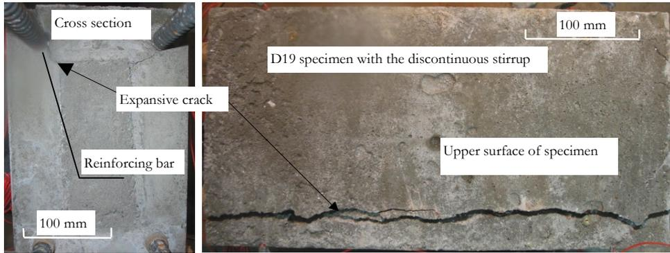
Figure 5: Extent of expansive crack in D19 specimen with discontinuous stirrup before the pull-out test.
