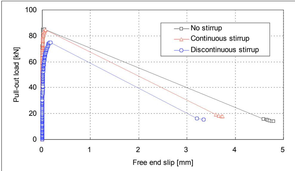
Figure 6: Relationship between pull-out load and free end slip in D19 specimens without expansive crack (the sound specimen).
