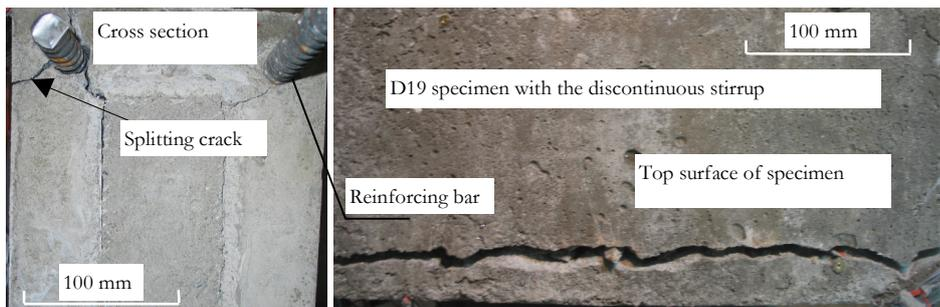
Figure 8: State of splitting crack after failure of the specimen.
