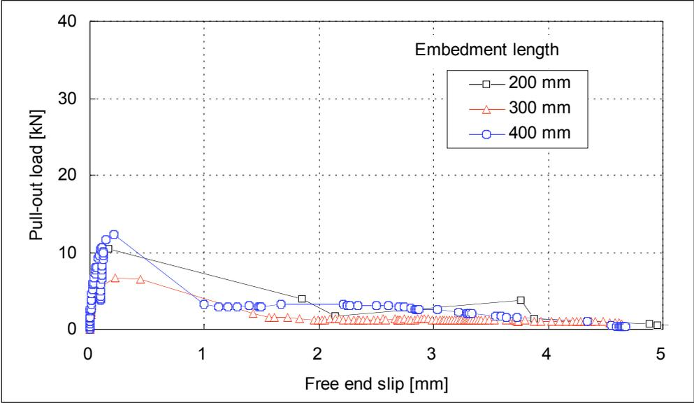
Figure 10: Relationship between pull-out load and free end slip in D10 specimens with the expansive crack.
