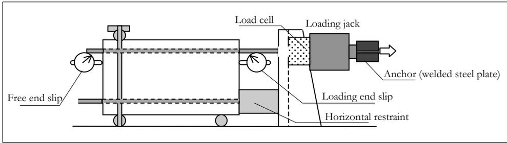
Figure 4: Pull-out test equipment.
