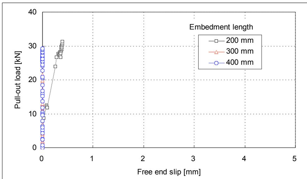
Figure 9: Relationship between pull-out load and free end slip in D10 specimens without expansive crack (the sound specimen).
