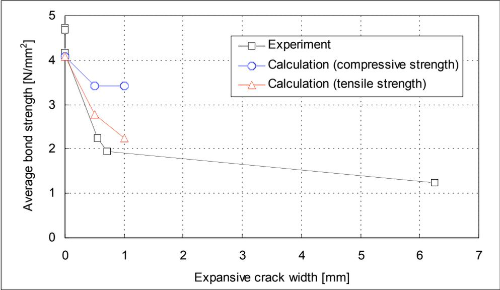
Figure 11: Relationship between calculated bond strength and expansive crack width, along with experimental bond strength.
