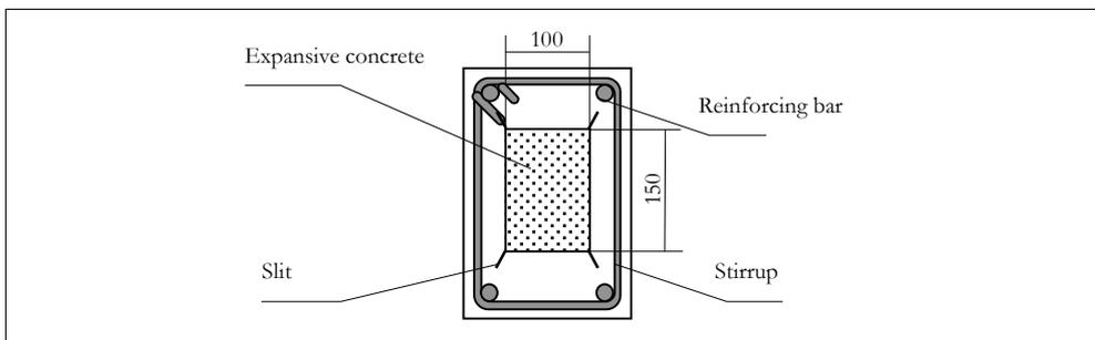
Figure 3: Cross-section of specimen, in which expansive crack was artificially induced using expansive concrete.
