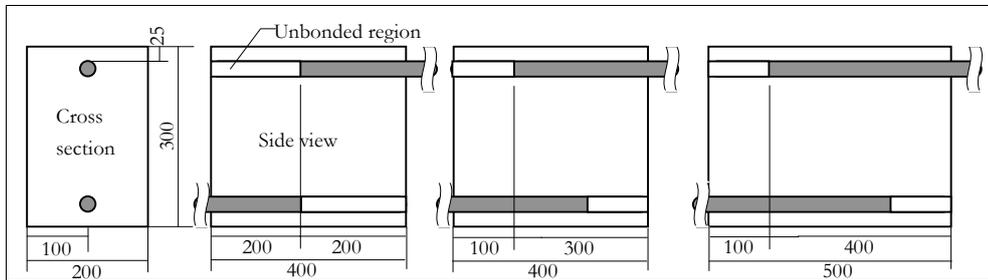
Figure 2: Shape and dimensions of the D10 pull-out type test specimen (dimensions in mm).
