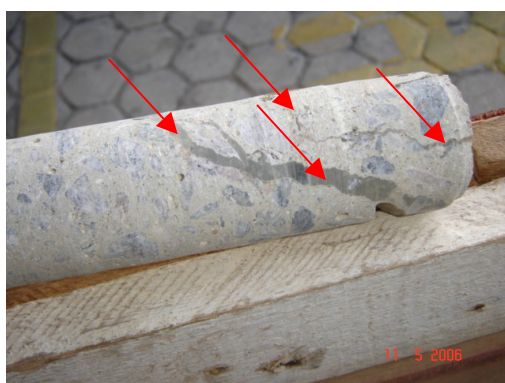
Figure 9: Specimen taken after washing of cracks showing the inner face of the crack free of material originating from the embankment.
