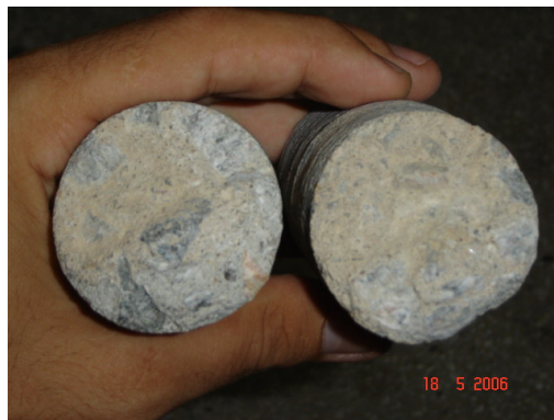
Figure 9: Specimen taken after washing of cracks showing the inner face of the crack free of material originating from the embankment.
