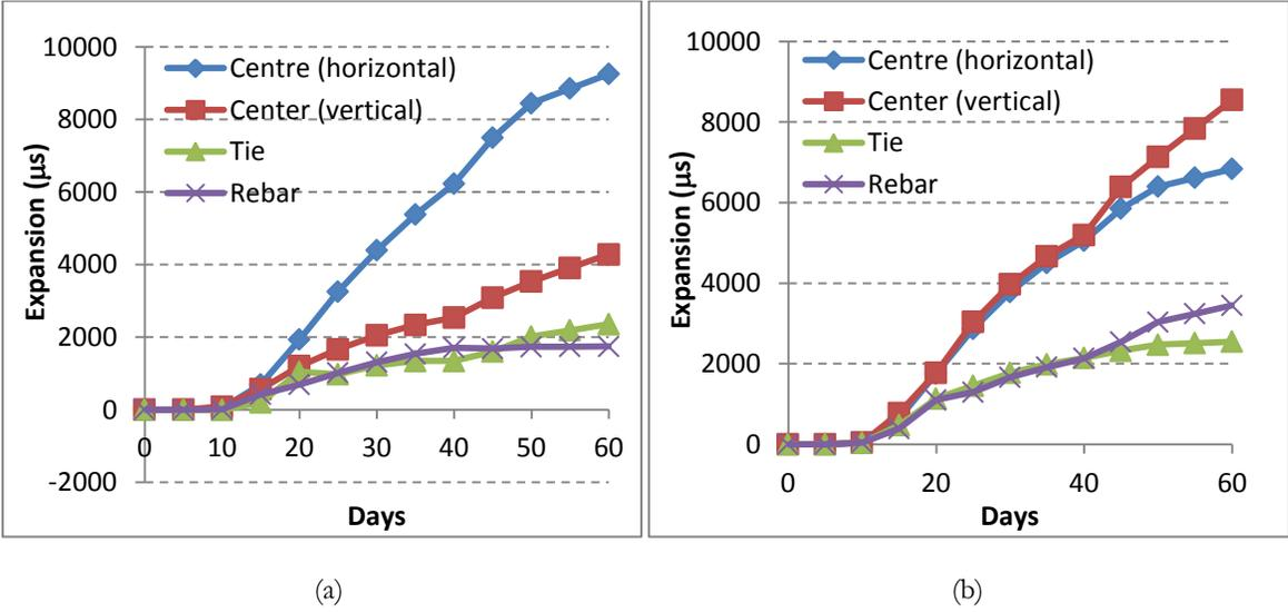
Figure 6: Strain development in the concrete and reinforcement steel in (a) circular column and (b) square column
