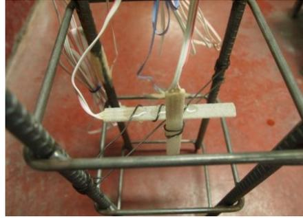
Figure 2: Arrangement for embedded gauges
