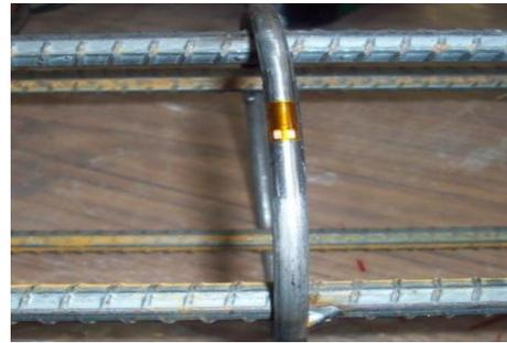
Figure 3: Insulated and normal strain gauges
