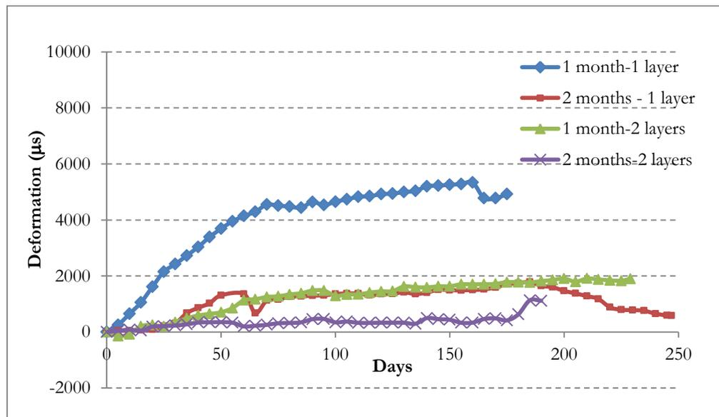
Figure 10: Deformation of CFRP wrap on the square columns
