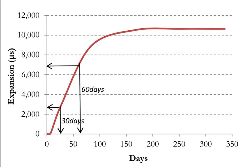
Figure 5: Free expansion measured on the concrete prism
