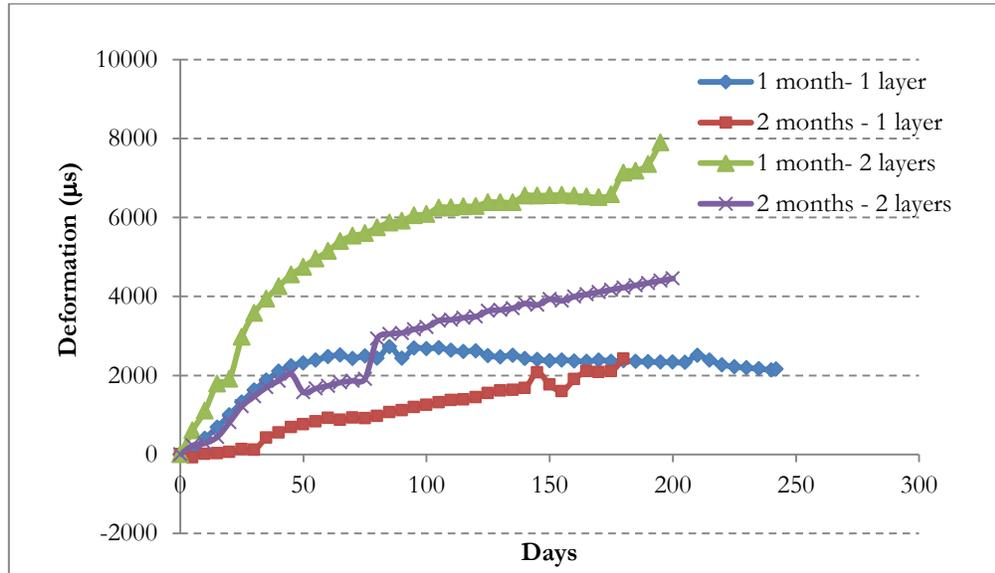
Figure 9: Deformation of CFRP wrap on the circular columns
