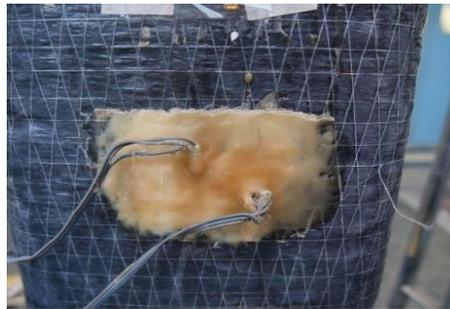
Figure 4: Exterior strain gauges with extra protection on fibre
