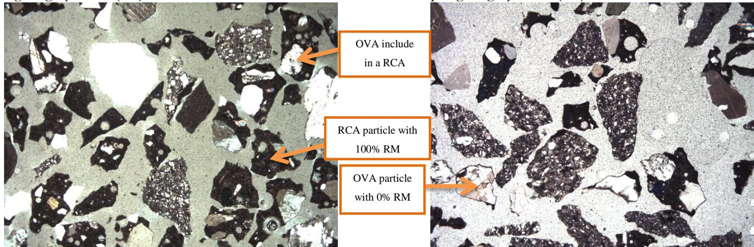
FIGURE 8: Micrographs (thin sections) of fine recycled aggregate particles (size fraction 1.18 - 0.63 mm).
