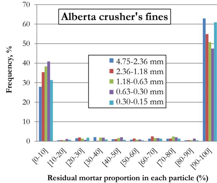
FIGURE 7: Frequency of particles incorporating different proportions of RM (in increments of 10%)
