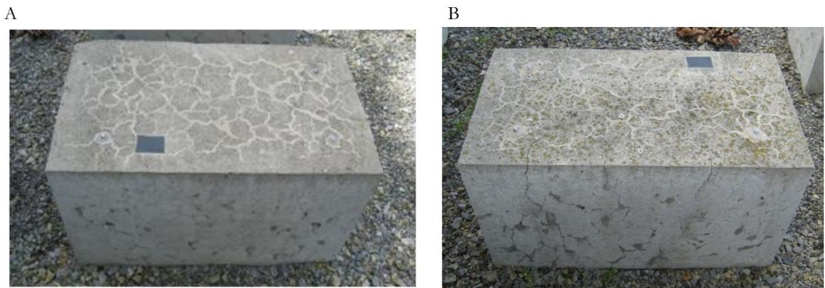
FIGURE 2: Exposure blocks incorporating the Alberta (A) and the Springhill (B) aggregates that were used for the manufacture of the RCA.
