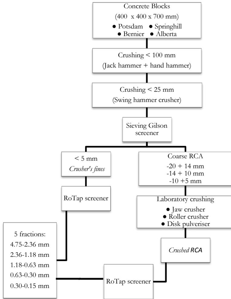
FIGURE 3: Description of the preparation of the RCA
