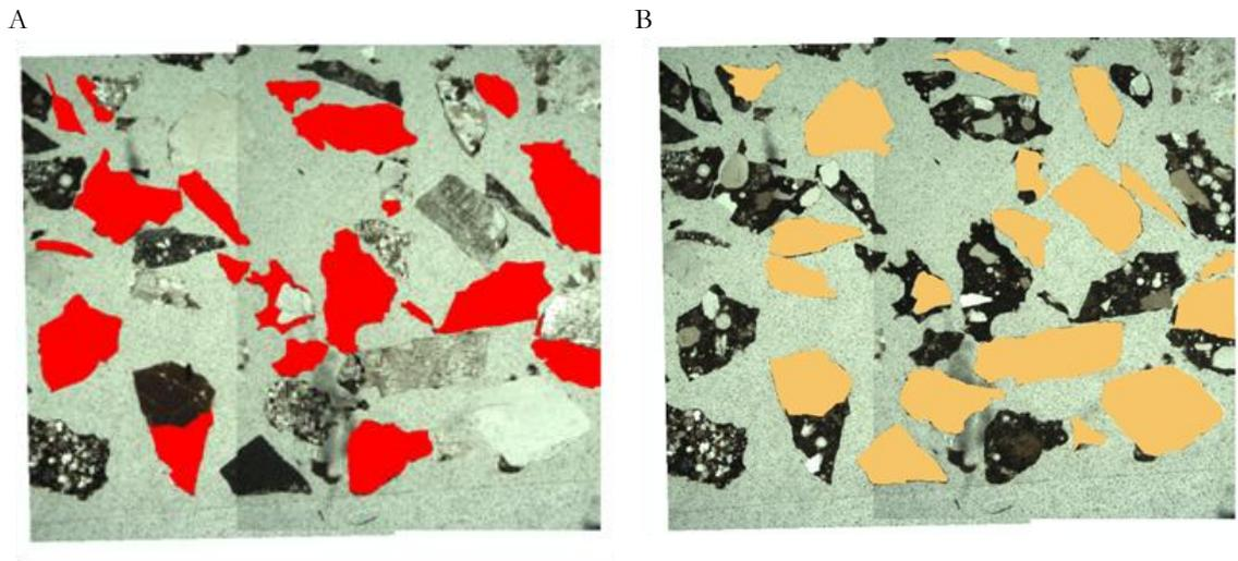
FIGURE 6: Example of segmentation of RCA particles (A) and OVA particles (B) for Alberta gravel (SG) (thin section incorporating aggregate particles of 2.36-1.18 mm in size). Only the particles appearing entirely on the picture are treated.
