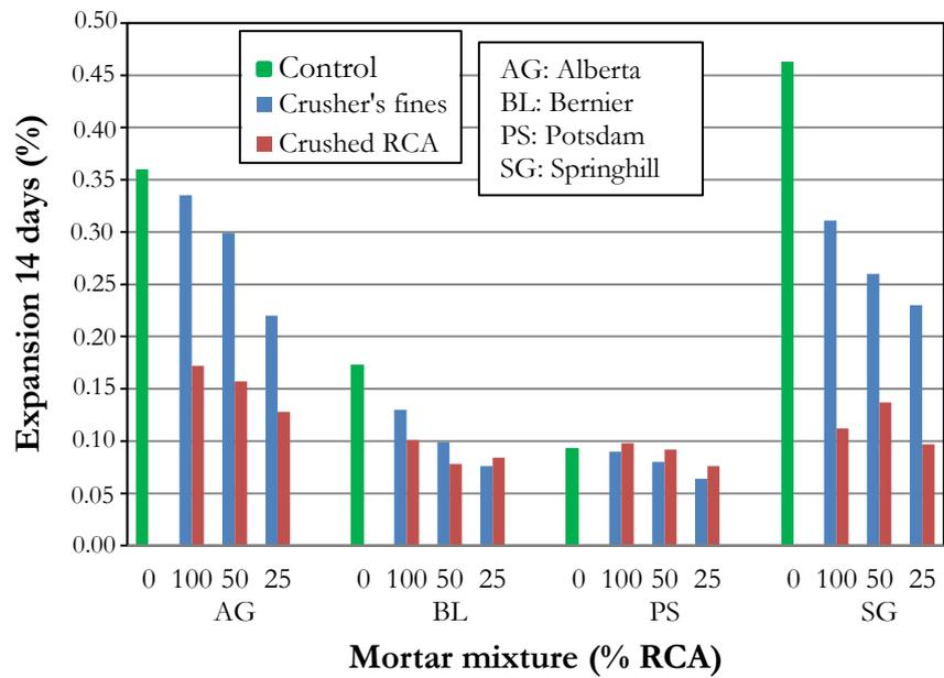
FIGURE 1: 14-day accelerated mortar bar expansions of the *crusher's fines* and the *crushed RCA* incorporating the four OVA selected for this study.
