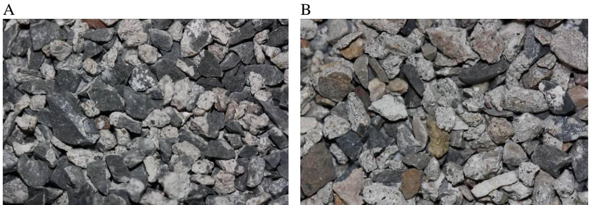
FIGURE 4: RCA incorporating the AG (A) and SG (B) aggregates (14-20 mm size fraction)
