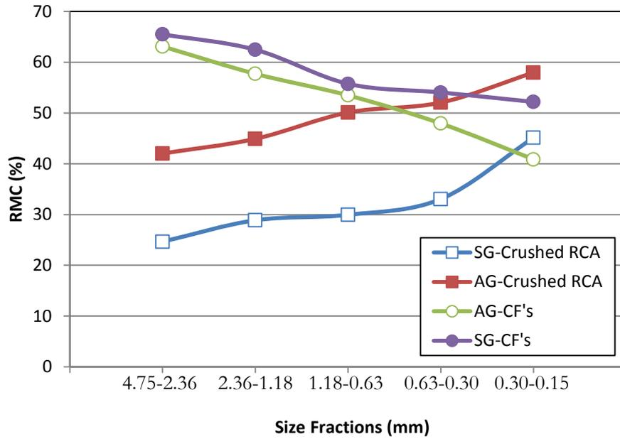
FIGURE 5: Total residual mortar content for the different particle sizes of the crushed RCA and crusher's fines (AG: Alberta gravel; SG; Springhill greywacke).
