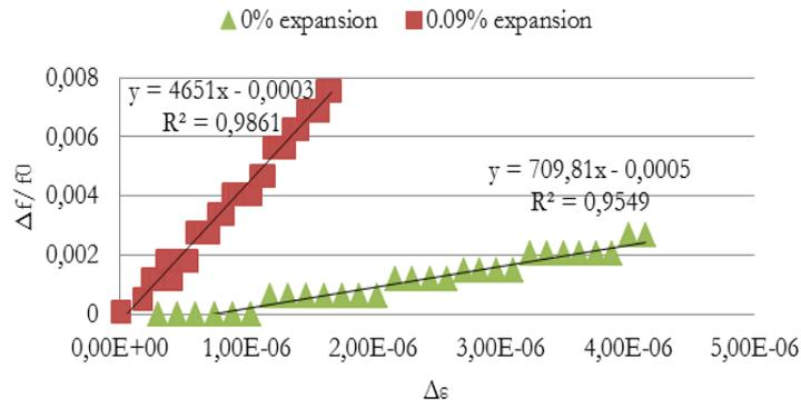
FIGURE 5: Determination of  $\alpha$  value for sample n°3 at 0% and 0.09% expansion
