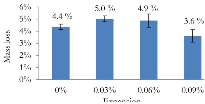
FIGURE 4: Evolution of the mass loss of reactive silica during TGA with expansion
