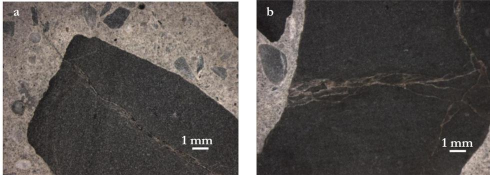
FIGURE 2: Typical petrographic features observed for 0.06% expansion (a) and 0.09% expansion (b)
