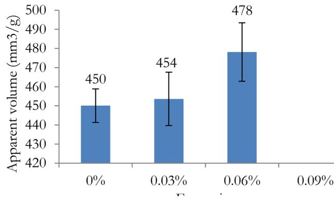
FIGURE 3: Evolution of the apparent volume of reactive silica with expansion
