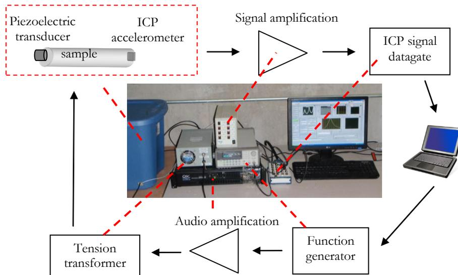
FIGURE 1: Experimental device for non linear resonance tests
