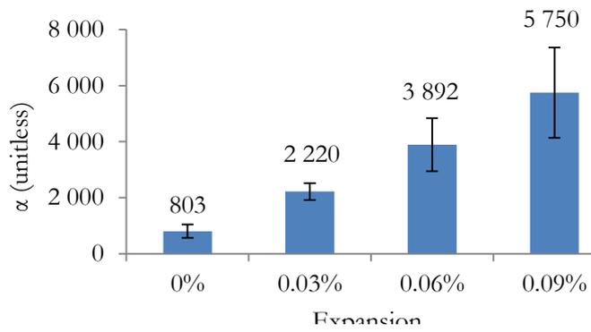
FIGURE 6: Evolution of nonlinear parameter  $\alpha$  with expansion
