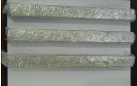
FIGURE 1: Mortar bars wrapped in plastic film.
