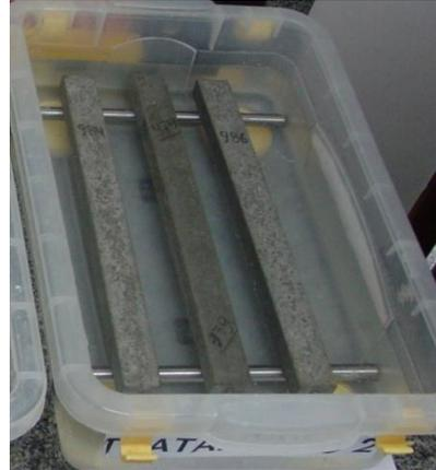
FIGURE 2: Immersion in deionized water.
