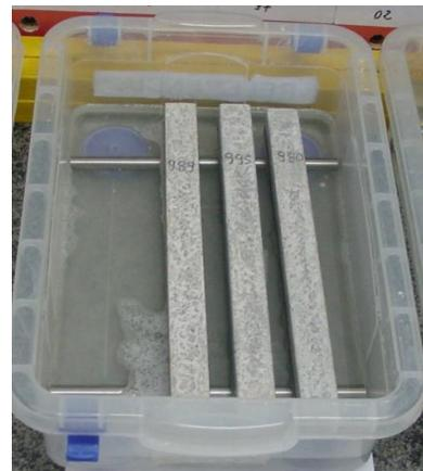
FIGURE 4: Surface saturation in lithium.
