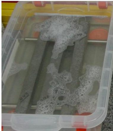
FIGURE 3: Total saturations in lithium.
