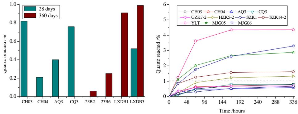
(a) 4-8mm crushed aggregates in the microbars (b) Less than 0.080mm powders in alkali solutions
