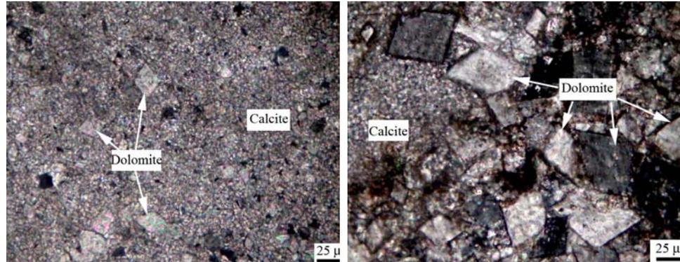
Fig. 2 Typical microstructures of the dolomitic limestones
