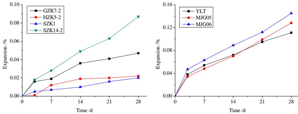
Fig. 4 Expansions of RILEM AAR-5 concrete microbars with 4-8mm crushed rocks GZK7-2, HZK5-1, SZK1, SZK14-2, YLT, MJG05 and MJG06
