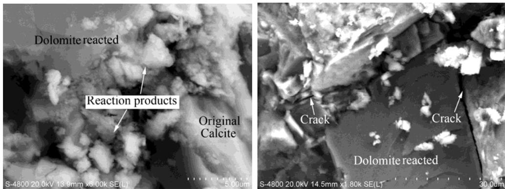
Fig. 7 Reacted dolomite, reaction products and cracks induced in dolomitic limestone aggregates of concrete microbars cured in 1.0 mol/l NaOH solutions at 80°C for 28 days
