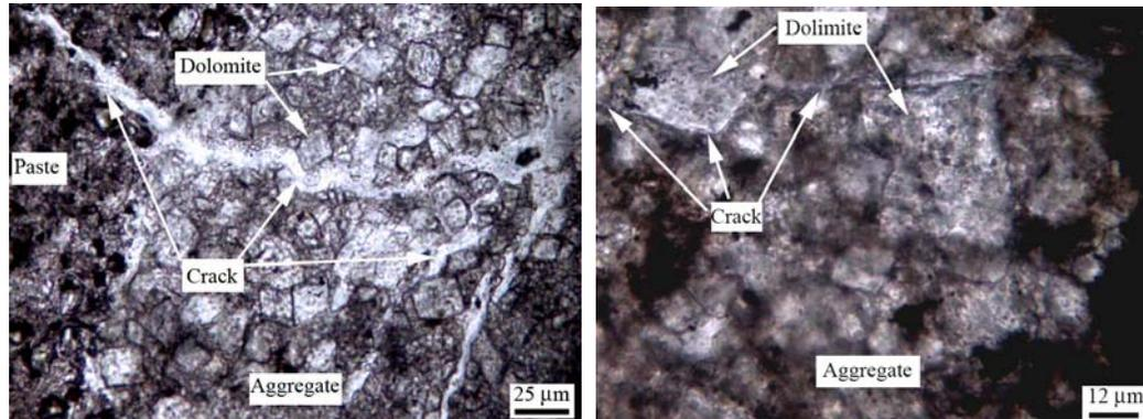
(a) Crack in aggregate CH03 and paste
