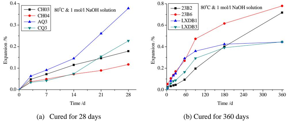
Fig. 3 Expansions of RILEM AAR-5 concrete microbars with 4-8mm crushed rocks CH03, CH04, AQ3, CQ3, 23B2, 23B6, LXDB1 and LXDB3
