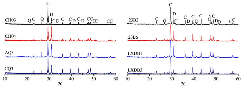
Fig. 1 XRD patterns of powders of rocks CH03, CH04, AQ3, CQ3, 23B2, 23B6, LXDB1 and LXDB3
