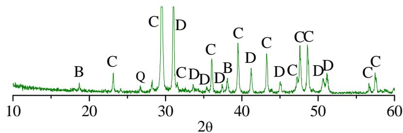
Fig. 8 XRD pattern of powdered dolomitic limestone 23B6 derived from concrete microbars cured in 1.0 mol/l NaOH solutions at 80°C for 360 days
