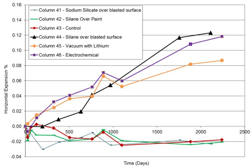
FIGURE 4: Expansion of moderately damaged bridge columns after treatments
