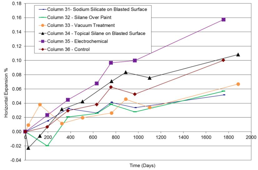
FIGURE 3: Expansion of moderately to severely damaged bridge columns after treatments
