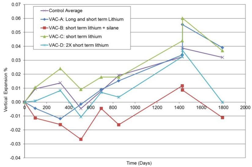
FIGURE 6: Expansions of vacuum treated jersey barriers
