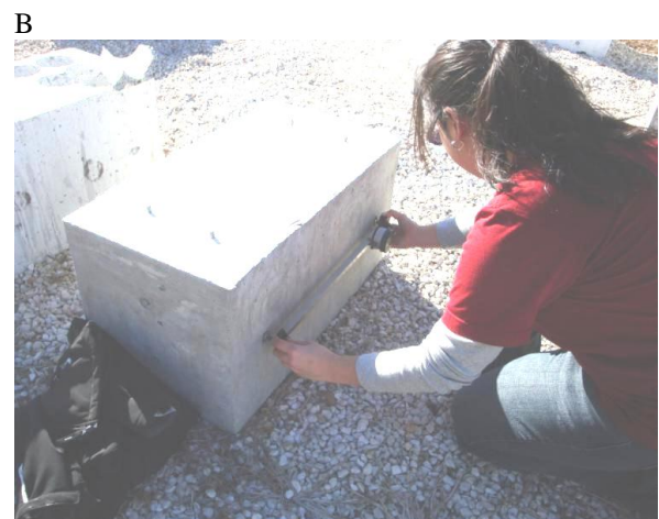
Figure 1: A. Exposure blocks on the outdoor exposure site at the University of Texas at Austin, USA. B. Expansion measurements of the exposure blocks.
