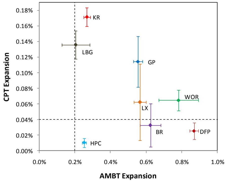
Figure 5: Comparison of expansions in the CPT and the AMBT with error bars showing standard deviation
