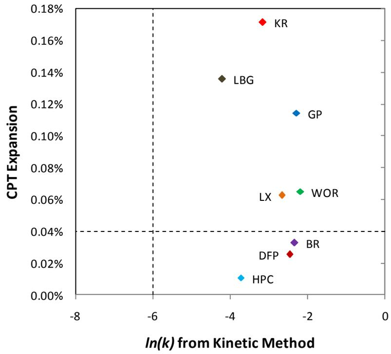
Figure 6: Comparison of critical limits in the CPT and the Kinetic Method
