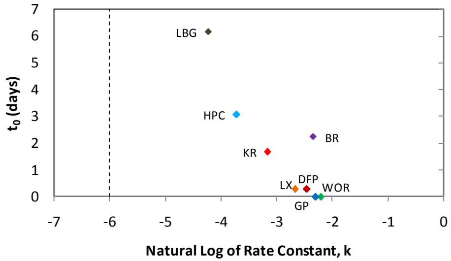
Figure 4:  $t_0$  vs.  $\ln(k)$  for eight aggregates analyzed using the Kinetic Method
