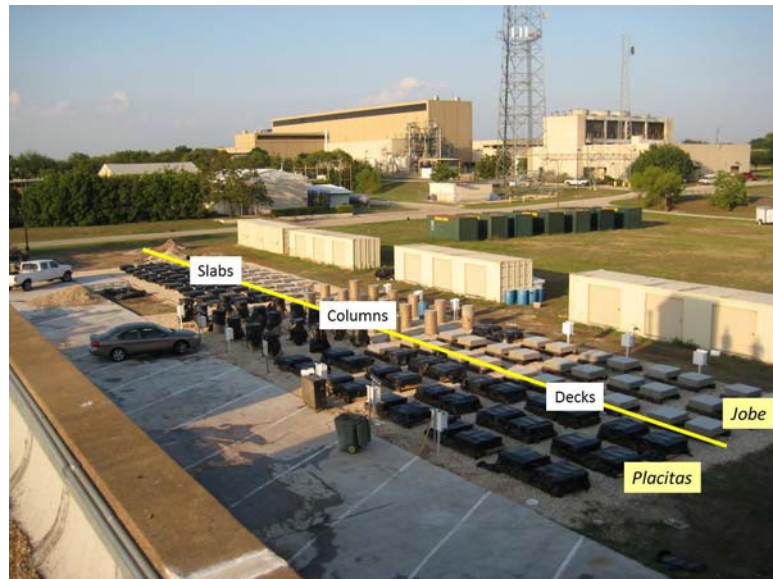
FIGURE 1: Photo of the outdoor exposure site in Austin, TX, showing the two reactive aggregates used (Jobe sand and Placitas gravel) and the three element types (slabs, columns, and decks)
