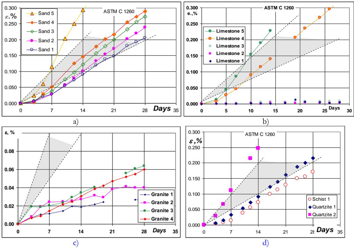
Figure 1 - Results of ASTM C 1260 for sands (a), limestones (b), granites (c), quartzites and schist (d) . Portuguese aggregates.
