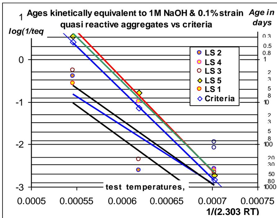
Figure 2 - Arrhenius plot for results of ASTM C 1260, ASTM C 227 and NF P18-590 tests with same sand (upper), and limestone (lower) aggregates tested in Figure 1, in comparison with same tests estimated from quasi reactive criteria in Figure 1, represented as filled diamonds. The regression and correlation coefficients obtained for the respective lines are presented in Table 3.
