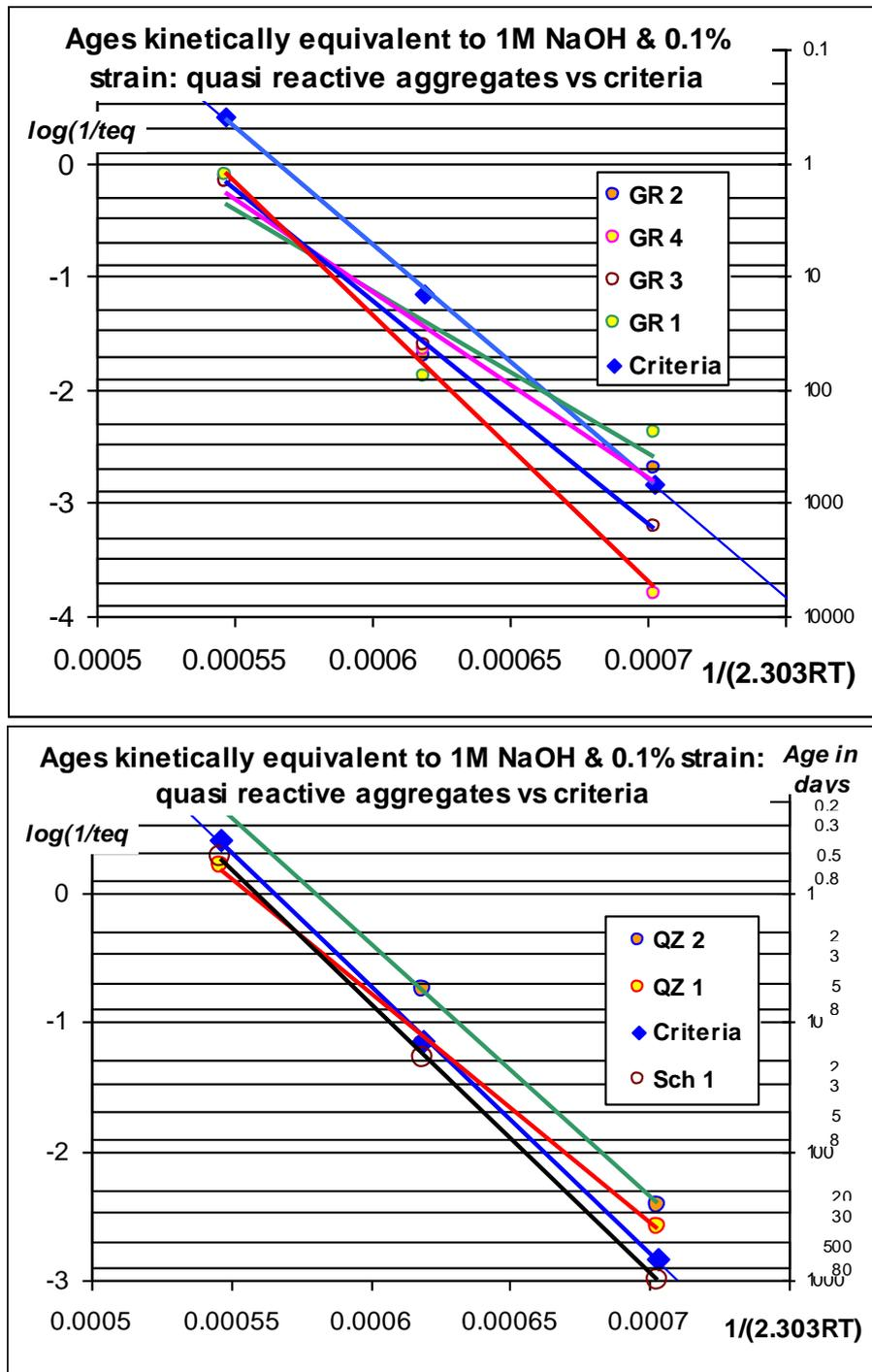
Figure 3 Arrhenius plot for results of tests ASTM C 1260, ASTM C 227 and NF P18-590 with same four granite (upper) and 2 quartzite and one schist (lower) aggregates tested in Figure 1, in comparison with same tests estimated from quasi reactive criteria from Figure 1, represented as filled diamonds. The regression and correlation coefficients obtained for the respective lines are presented in Table 3
