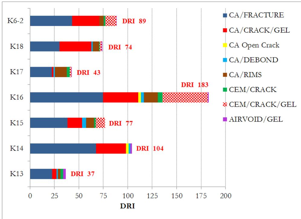
FIGURE 3c: DRI's of a series of concrete prisms made from different layers of the Pittsburgh quarry. Prism K6-2 was made from the stockpile that presumably represents the average of all the layers with a DRI of 86.
