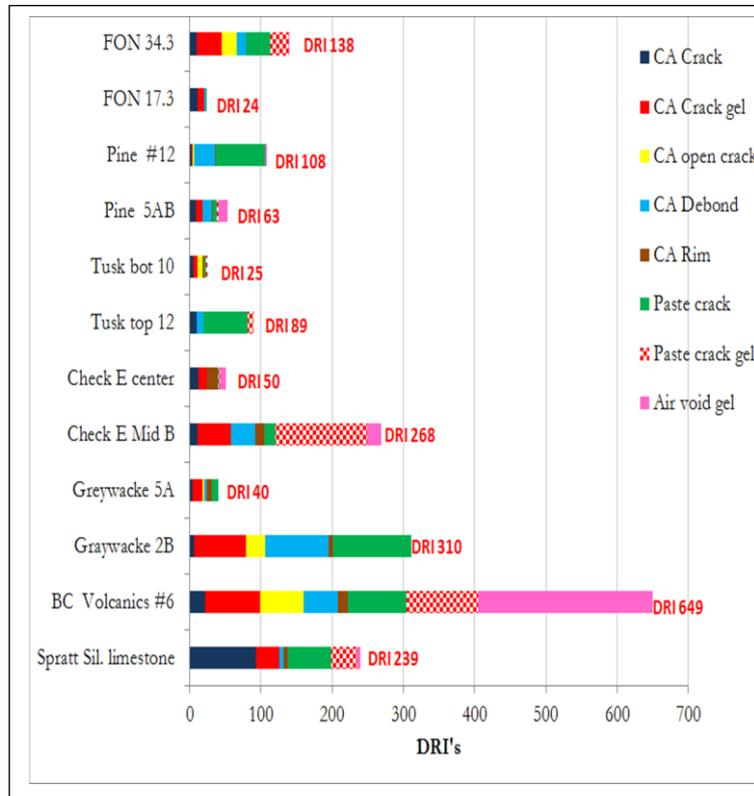
FIGURE 2: DRI chart showing variations in the DRI's of assorted cores, affected by ASR, taken from various parts of structures and of cores containing different types of aggregates.
