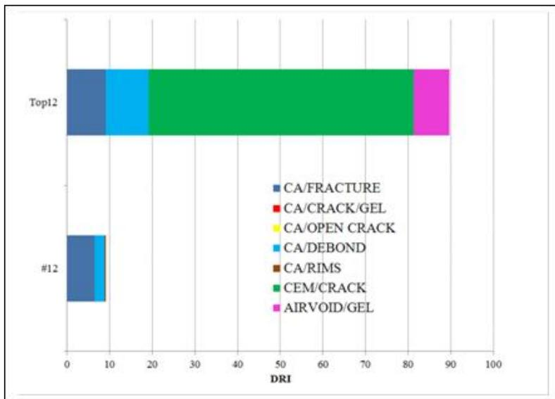
FIGURE 4: Chart of DRI's of two cores, one taken near the top (Top12) and the other at depth. Note there is some evidence of ASR in the form of gel in air voids.
