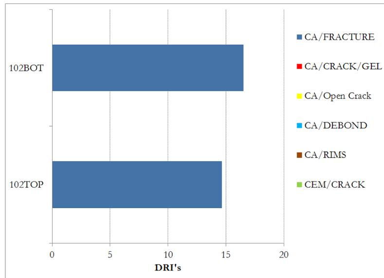
FIGURE 6: DRI chart of two cores taken from near the top and bottom of an airport runway that only exhibits cracking in the coarse aggregate particles.
