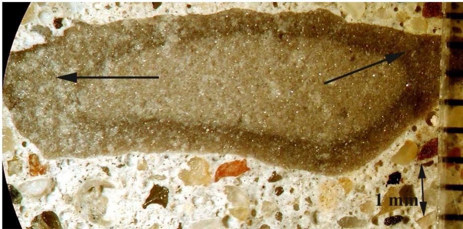
FIGURE 3b: Photograph of a wide reaction rim around a particle of dolomitic limestone. The arrows point to the rim. Scale divisions are in mm.
