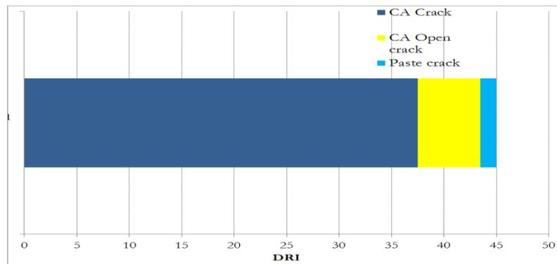
FIGURE 1: Chart of the DRI of a concrete cylinder, made with a non-reactive limestone aggregate, and cured for 3 months in a fog room.
