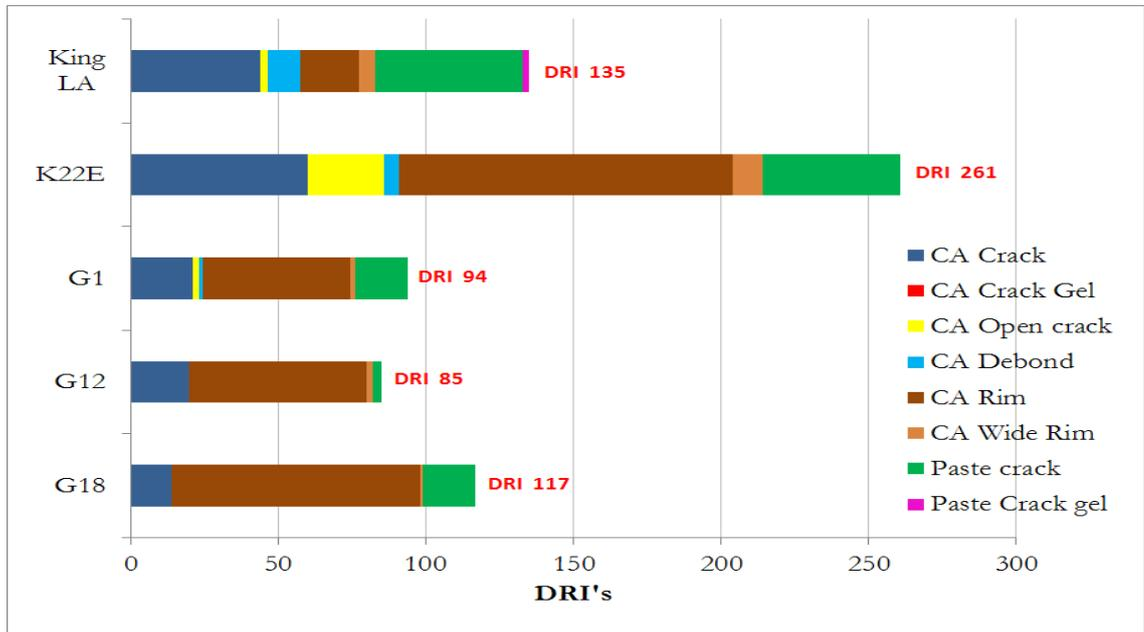
FIGURE 3a: Chart of the DRI's of assorted concrete cores affected by ACR. The core King LA that contains some gel in cracks in the cement paste was taken from, an experimental sidewalk in Kingston Ontario. The concrete was made with low alkali cement. Note the presence of wide reaction rims.
