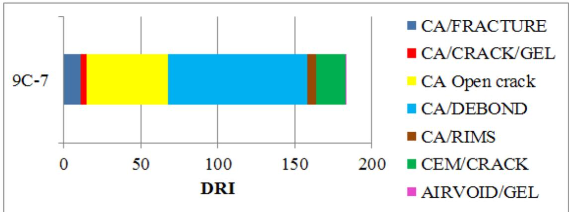
FIGURE 5a: DRI of a core from a bridge in Texas showing extensive debonding around coarse aggregate particles that is characteristic of concrete affected by DEF. Note that there is gel in some cracks in coarse aggregate particles indicating that ASR is occurring along with DEF.
