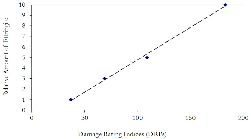
FIGURE 5c: Graph showing the correlation between the amount of ettringite in the concrete and the DRI's.
