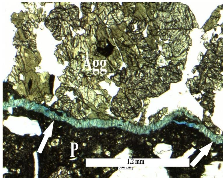
FIGURE 5b: Photograph of a thin section viewed in natural light showing compacted ettringite needles filling a crack at the paste aggregate interface (debonding) indicated by arrows. The blue color is due to blue epoxy used to impregnate the thin section.
