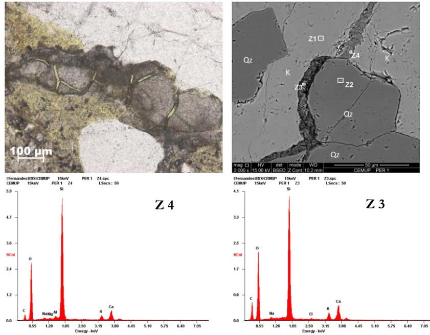
FIGURE 3: Upper image: Brownish ASR-gels formed *in situ* on medium grained granitic gneiss (plane polarised light) and within granitic gneiss (SEM backscatter). Rosette-like gel (Z3) and dense gel (Z4) on grain boundaries with quartz and microcline (K). Notice the apparent dissolution of feldspar near Al bearing Z4. Core A- Per 1.
