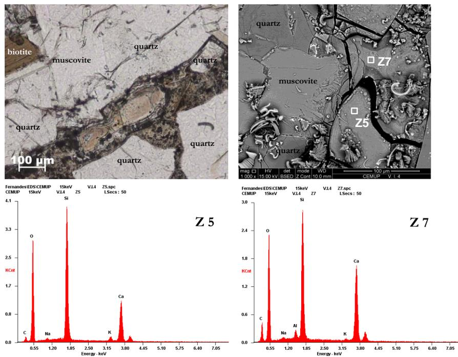
FIGURE 1: ASR-gel (Z5, Z7) formed *in situ* in contact with muscovite and medium grained quartz (1500 μm). Plane polarised light and SEM backscatter. The curved and branched deposits represent calcium carbonate which had grown from gel (old thin section). Core V-1.
