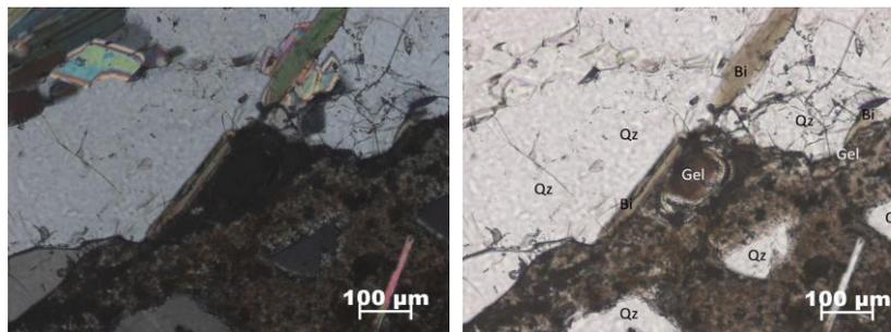
FIGURE 2: Brown ASR-gels formed *in situ*, typically coinciding with presence of biotite. The adjacent quartz (ca. 1000 μm) was strain free and in optical continuum, exhibited parting. Left: cross polarised light, right: plane polarised light. Sample V1.
