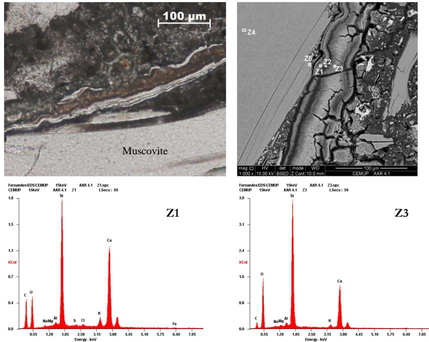
FIGURE 5: Upper left: ASR-gel in the interface with the cement paste close to a muscovite crystal (plane polarised light). Upper right: Backscatter image showing ASR gel with a zoned structure. Analysed gels (Z1 and Z3) refer to the EDS spectra below. Sample AAR-4.
