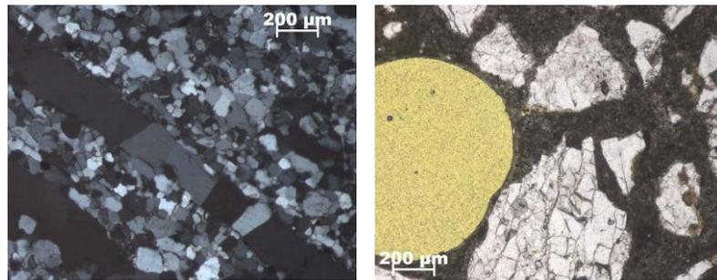
FIGURE 6: Innocuous Norwegian mylonite, sample 275. Left image (crossed polarised light) shows the annealed texture, with much quartz < 100 μm. Right image (plane polarised light) shows lack of ASR-gel formation after 14 days exposure according to AAR-2. Notice the typical scarcity of mica and accentuated grain boundaries.
