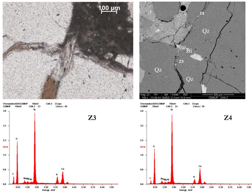
FIGURE 4: ASR-gel occurring within coarse quartz (Qz) with micro cracks converging to a biotite crystal (Bi). Plane polarised light and backscatter image. Analysed gels (Z3 and Z4) refer to the EDS spectra below. Concrete from the wall of an energy dissipation basin (CAA).
