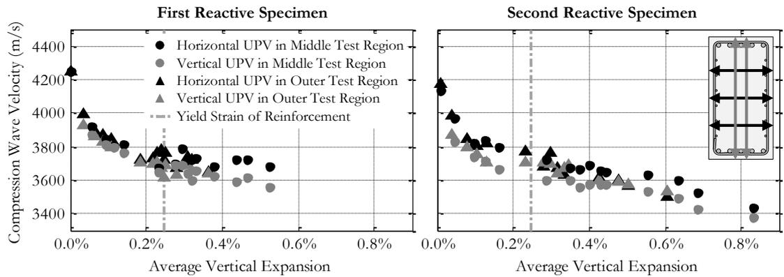
FIGURE 4: Results from UPV testing on the two reactive beam specimens. The compression wave velocity in the nonreactive specimen varied between 4225 and 4370 m/s over the monitoring period.
