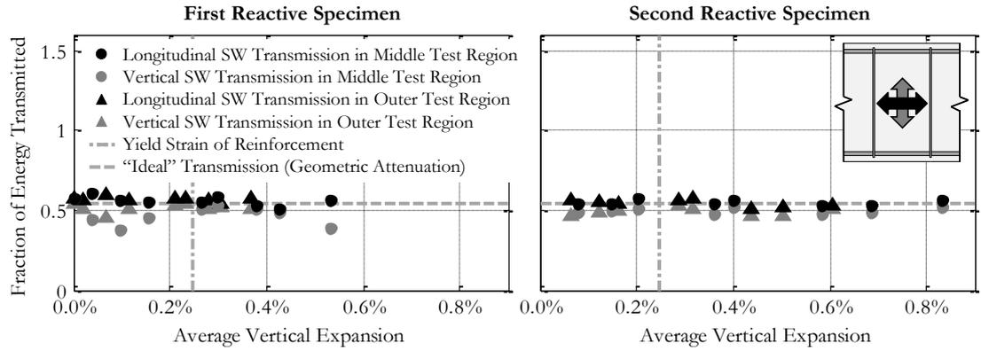
FIGURE 7: Results from SWT testing on the two reactive beam specimens. The fraction of SW energy transmission in the nonreactive specimen varied between 0.523 and 0.566 over the monitoring period. The “ideal” transmission includes only geometric attenuation of the point source-induced wave.
