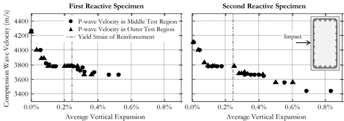
FIGURE 5: Results from impact echo testing on the two reactive beam specimens. The compression wave velocity in the nonreactive specimen varied between 4220 and 4390 m/s over the monitoring period.
