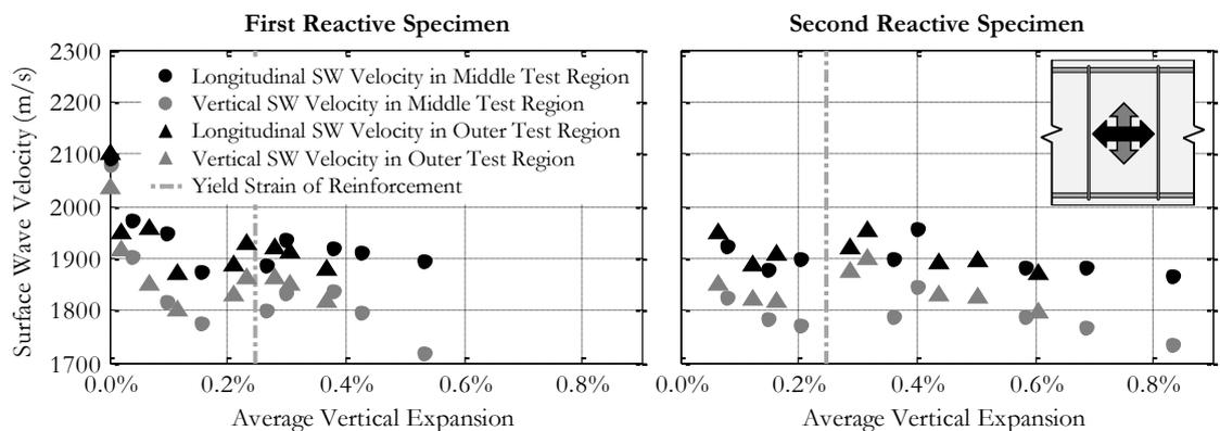
FIGURE 6: Results from SASW testing on the two reactive beam specimens. The surface wave velocity in the nonreactive specimen varied between 2020 and 2150 m/s over the monitoring period.
