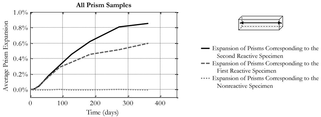
FIGURE 8: Results from expansion monitoring of the small prism samples cast alongside the large beam specimens. As with the beam specimens, larger and more rapid expansion was observed in the prisms corresponding to the second reactive specimen. This is likely due to higher curing temperatures.
