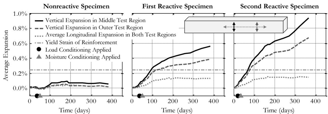
FIGURE 3: Results from expansion monitoring of the three beam specimens. The largest and most rapid expansions were observed in the vertical direction in the middle test region, where the reinforcement provides the least amount of restraint. The larger and more rapid expansions observed in the second reactive specimen are expected to be a result of the higher curing temperatures in this specimen.
