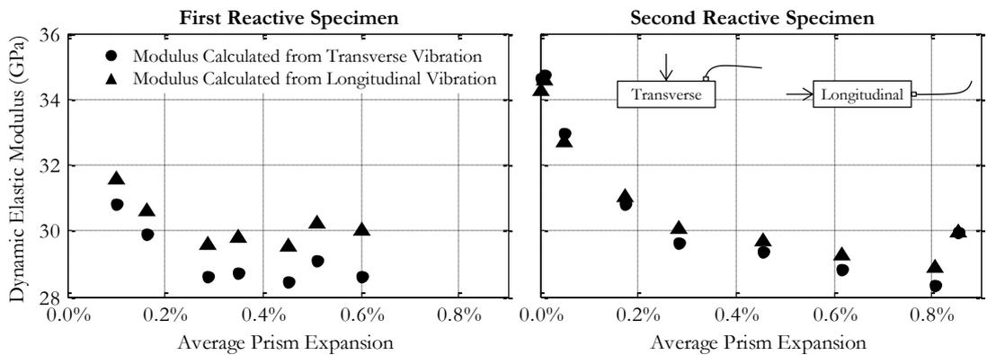
FIGURE 9: Results from resonant frequency testing of the reactive prism samples corresponding to the two reactive beam specimens. The dynamic modulus computed from the transverse and longitudinal vibration of the nonreactive prisms varied between 36.2 and 37.2 GPa over the monitoring period.
