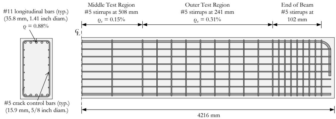
FIGURE 1: Geometry and reinforcement layout of the beam specimens. Note that the specimens are symmetric about the center line shown.
