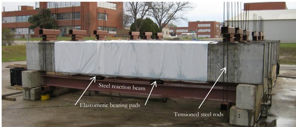
FIGURE 2: Specimens conditioning outdoors. Note the tarp wrapped around the specimens to trap in the moisture. The steel beam, tubes and rods are used to apply the simulated service load.
