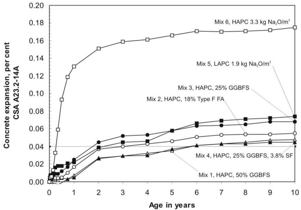
FIGURE 2: Expansion of concrete prisms in the laboratory at 38°C.
