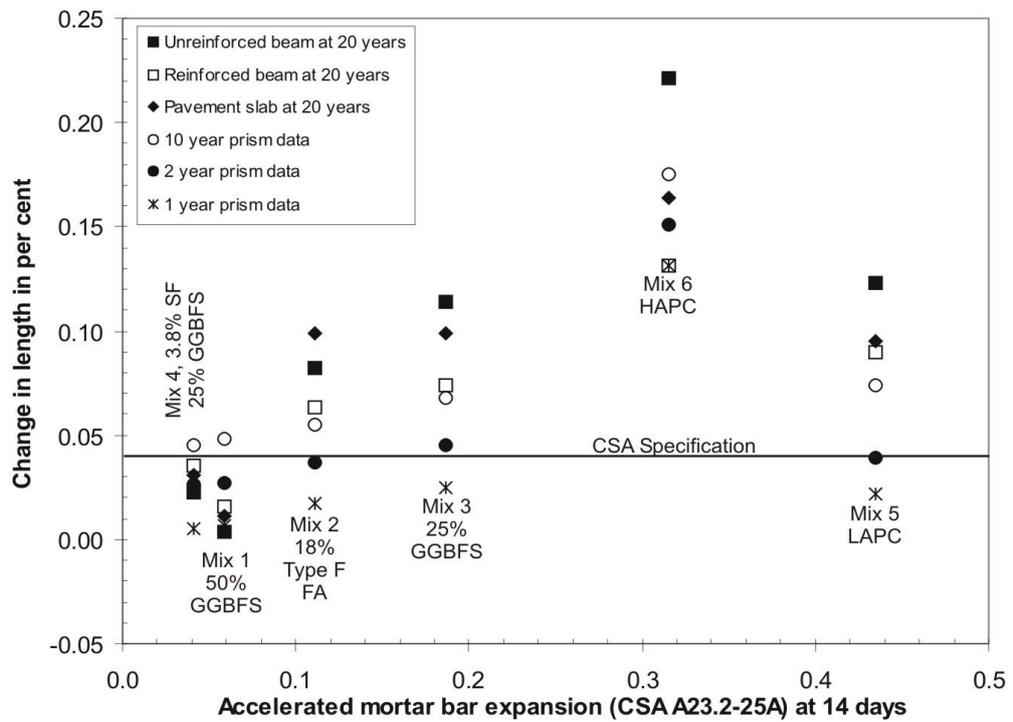
FIGURE 7: Mortar bar expansion versus concrete field expansion at 20 years.
