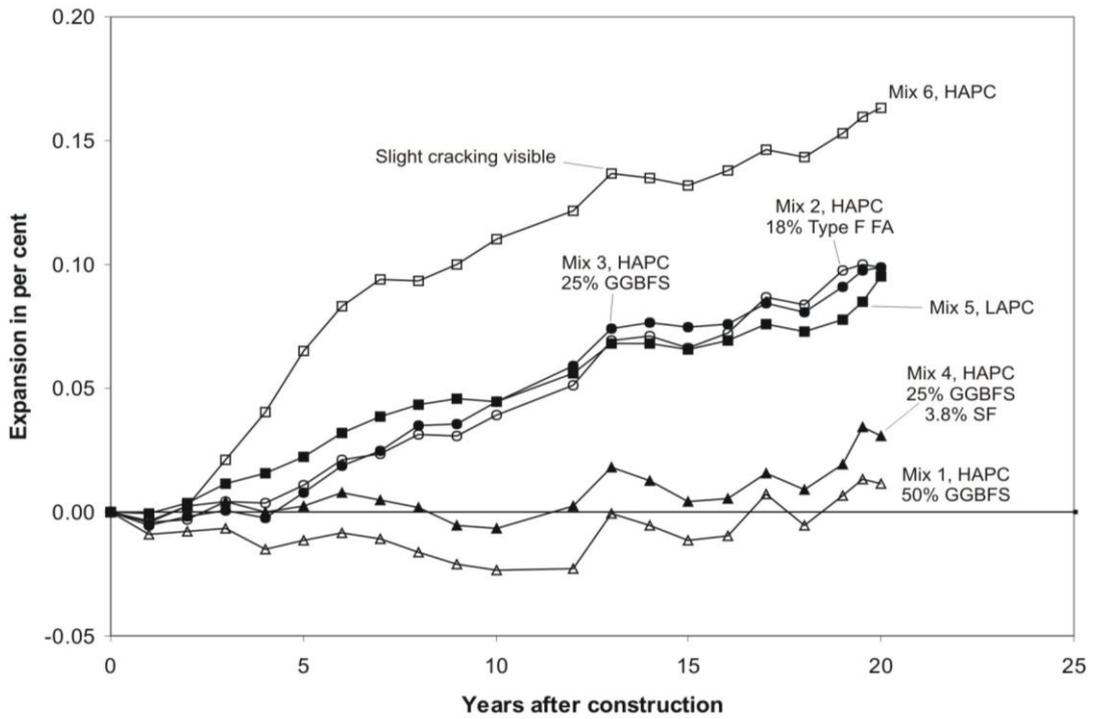
FIGURE 5: Expansion of outdoor exposed concrete pavement slabs
