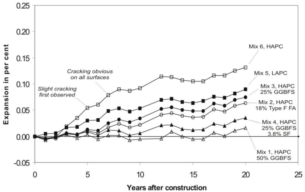
FIGURE 4: Expansion of outdoor exposed reinforced concrete beams.
