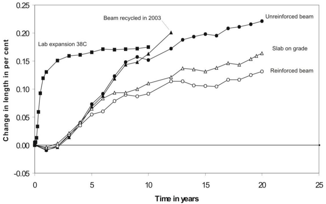
FIGURE 6: Expansion of mixture 6 (high-alkali cement) in various elements.
