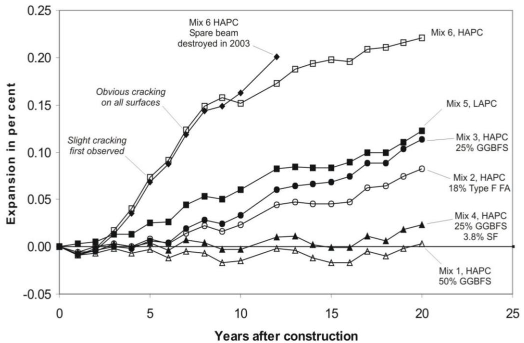
FIGURE 3: Expansion of outdoor exposed unreinforced concrete beams.
