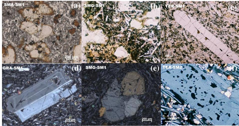
FIGURE 1: Photomicrographs of the volcanic aggregates studied: (a) Olivine with iddingsitized rims in SMA-SM1 sample (PPL); (b) Volcanic glass as an intergranular filler in SMG-SM1 sample (PPL), (c) Sanidine phenocrysts in TER-SM1 sample (PPL), (d) Zoned plagioclase in an intergranular groundmass in GRA-SM1 sample (XPL); (e) Clinopyroxene crystals in SMG-SM1 samples (XPL) and (f) Plagioclase phenocryst containing inclusions of andesitic glass in TER-SM2 sample (XPL).
