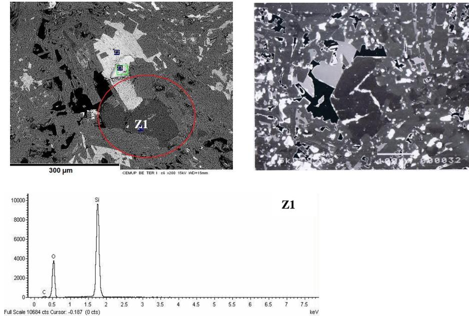
FIGURE 2: Silica in trachyte, presently microcrystalline quartz (TER-SM1): Irregular-shaped (left), and euhedral (right). SEM image and EDS spectrum [left, 23].
