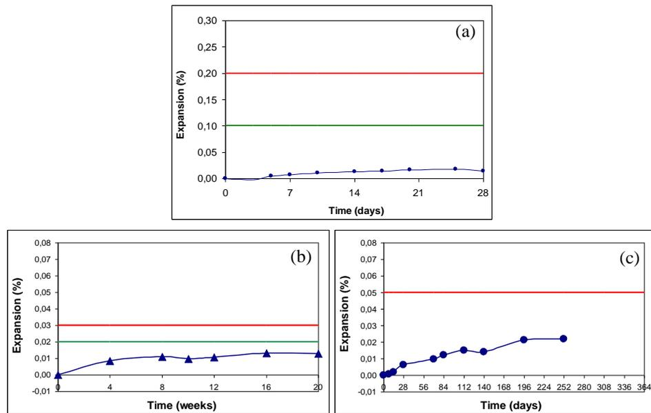
FIGURE 4: Expansivity test results of trachybasalt (SMG-SM1) sample [23]: a) ASTM C 1260-07; b) AAR-4; c) AAR-3.
