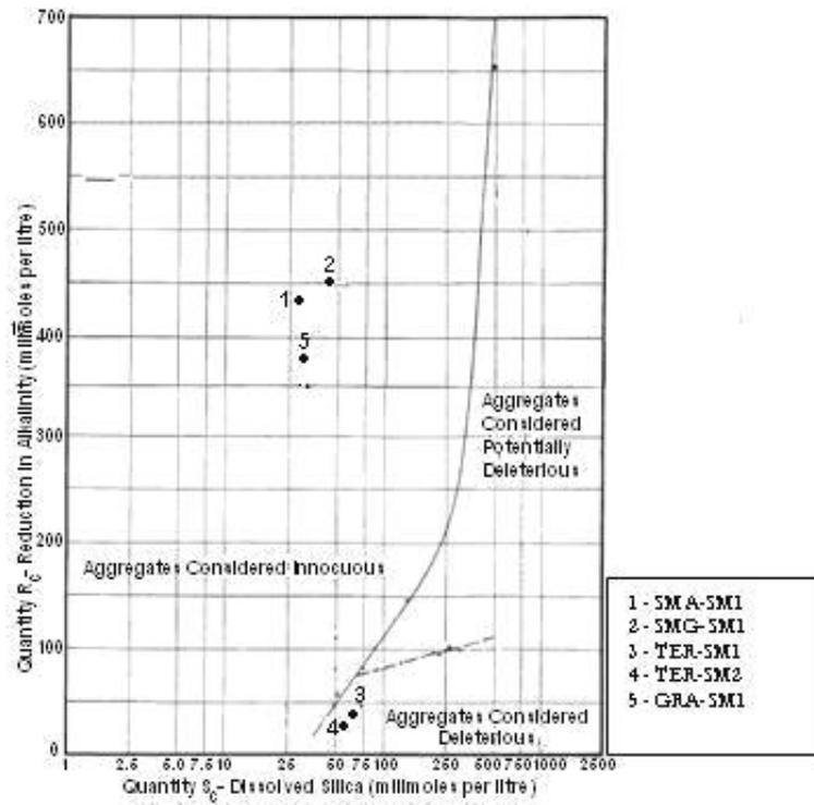
FIGURE 3: ASTM C 289-07 chemical test of basaltic rocks (1,2,4,5) and trachyte (3).
