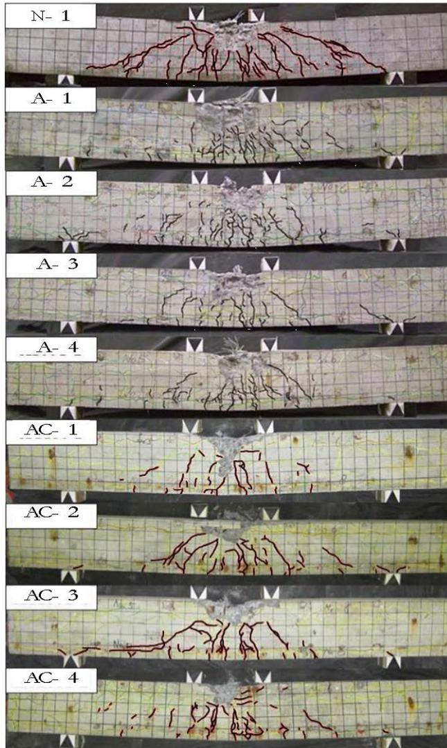
FIGURE 4: Final failure mode
