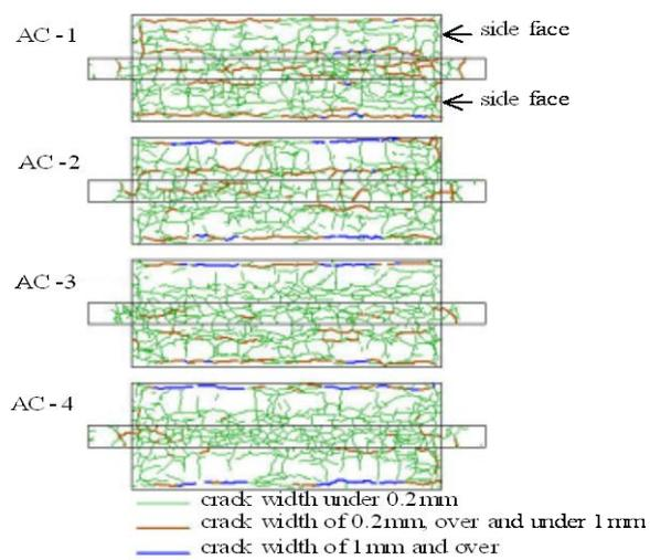
FIGURE 3: Condition of crack before loading tests
