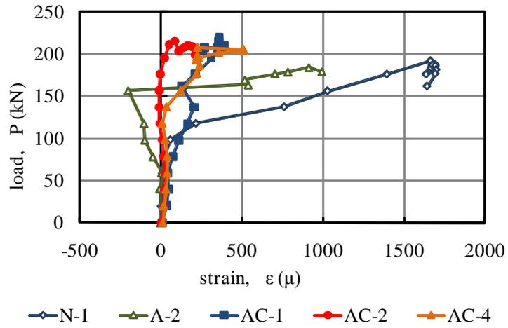
FIGURE 7: Relationship between load and strain of shear reinforcement
