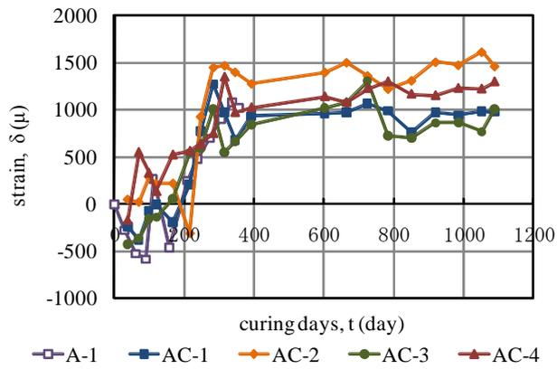
FIGURE 2: Axial strain of ASR expansion
