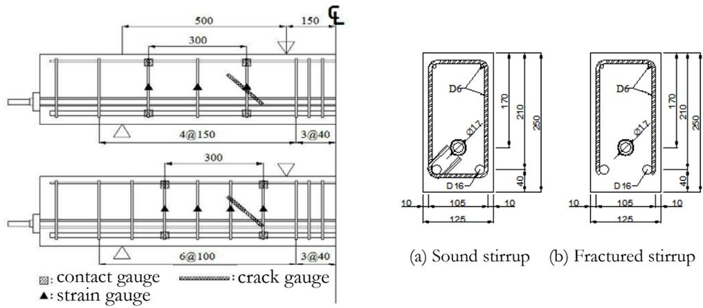
FIGURE 1: Dimensions of specimens and loading condition
