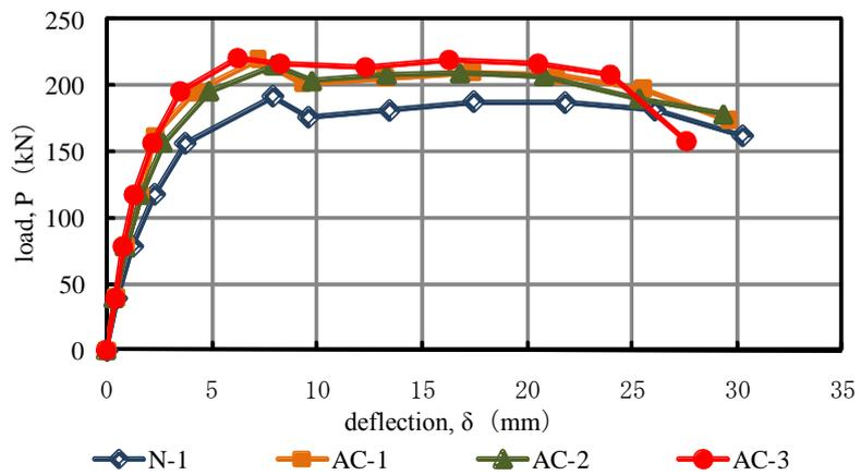
FIGURE 5: Relationship between load and deflection(AC-series and N-1)
