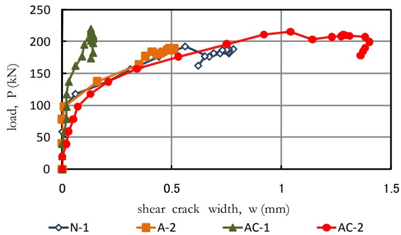
FIGURE 8: Relationship between load and shear crack width
