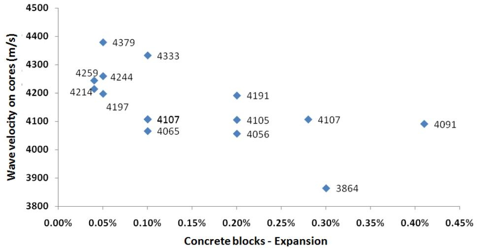
FIGURE 1: Correlation between ultrasonic pulse velocities measured on the cores and expansion of the concrete blocks and (all mixtures).
