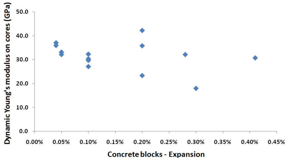
FIGURE 2: Relation between dynamic modulus of elasticity measured on cores and expansion of the concrete blocks (all mixtures)
