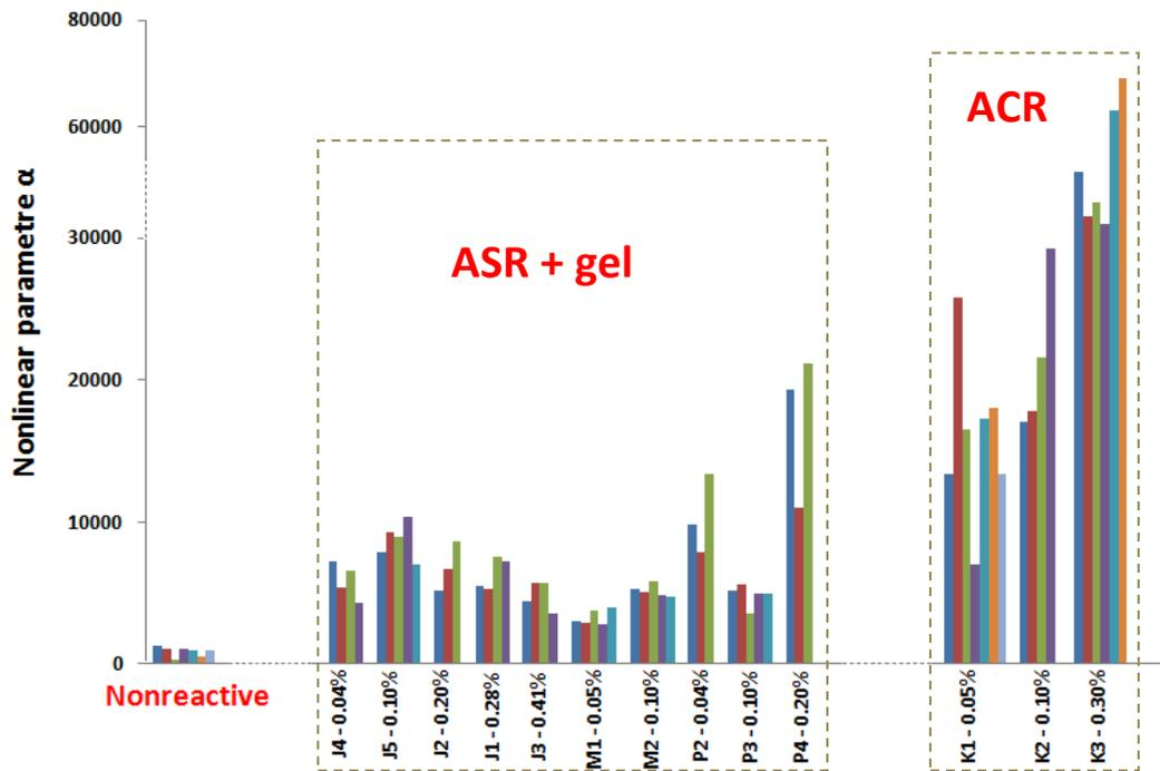
FIGURE 5: Frequency shift (nonlinear parameter  $\alpha$ ) for different aggregates with various degrees of reactivity. Expansion generally increases with expansion for every type of aggregate.
