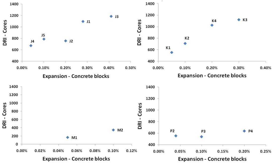
FIGURE 6: Relation between DRI of the cores and the expansion of the concrete blocks.
