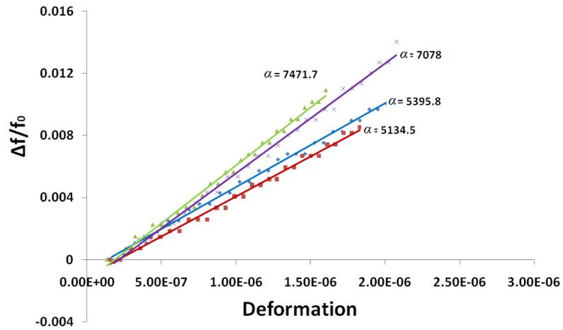
FIGURE 4: An example of the curve of resonant frequency shift – deformation for concrete cores made with cherty sand Jobe. The expansion of the concrete block was 0.28%. The unit of the deformation is (m/m).
