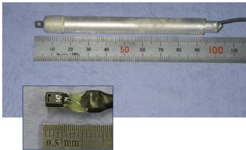
FIGURE 3: Temperature-humidity sensor
