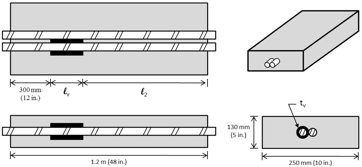
Figure 3: Specimen geometry for lap-splice sample
