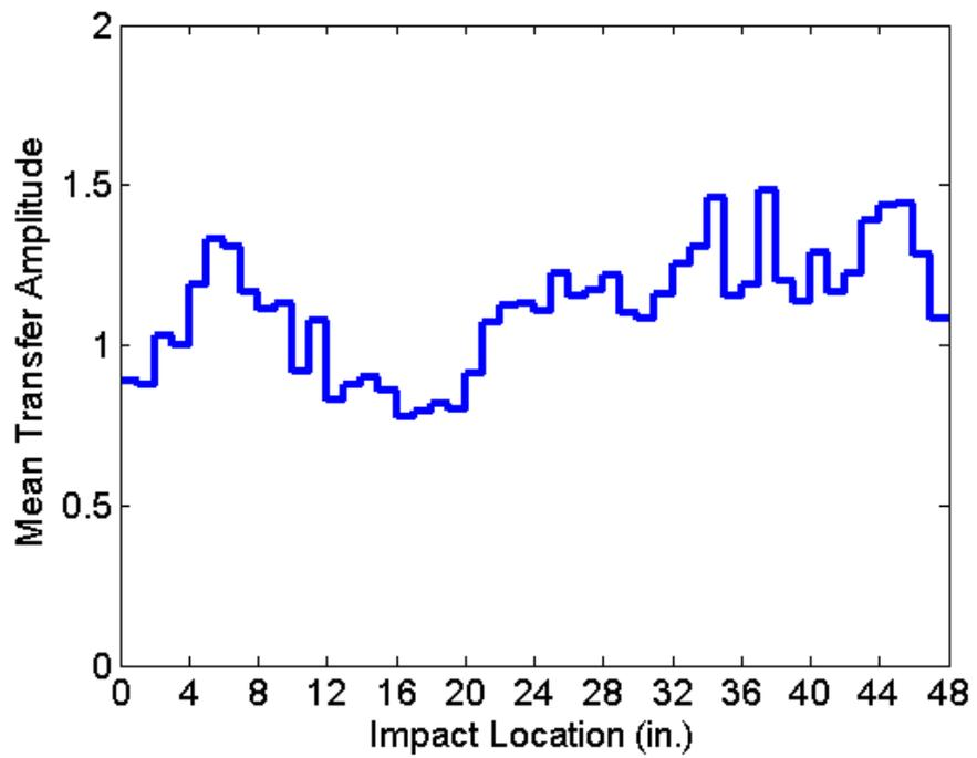
Figure 8: Mean transfer amplitude over predicted steel frequencies along Sample 2
