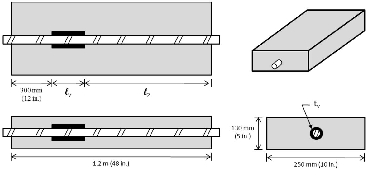
Figure 2: Specimen geometry for control sample
