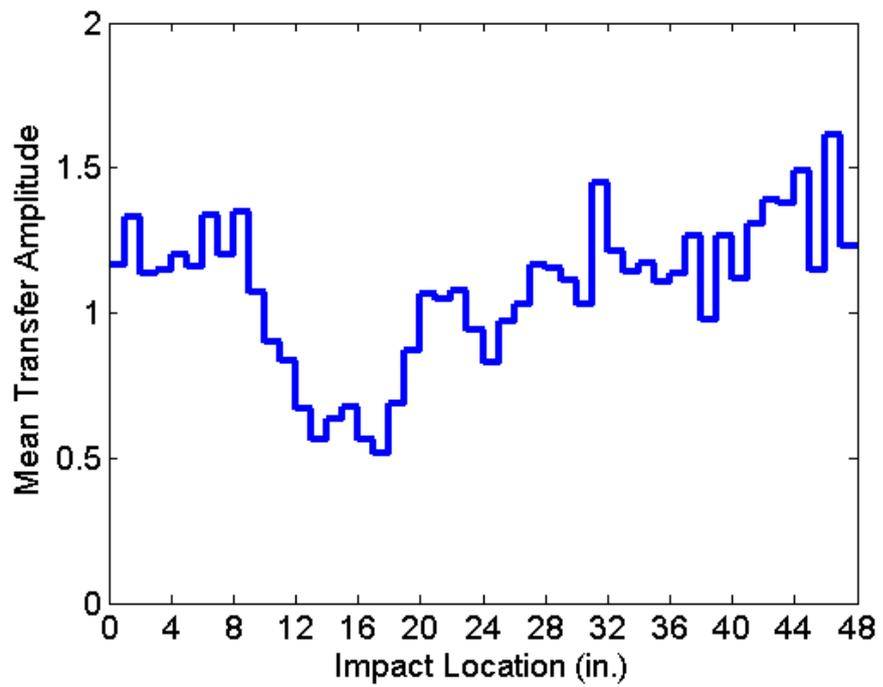
Figure 6: Mean transfer amplitude over predicted steel frequencies along Sample 1
