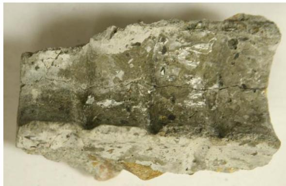
Figure 1: A portion of a core removed from an ASR-affected structure showing cracking parallel to the main reinforcement. Petrographic analysis of this specimen shows ASR gel (white areas) at the steel concrete interface.
