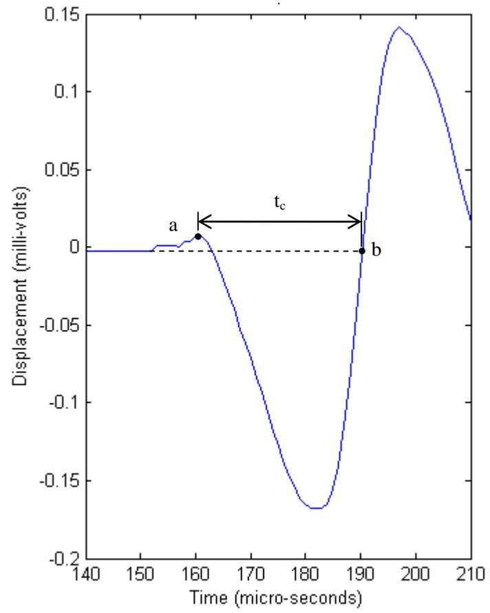
Figure 4: Typical R-wave with measured contact time
