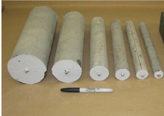
Figure 1: Photograph of specimens that were used for length change measurement
