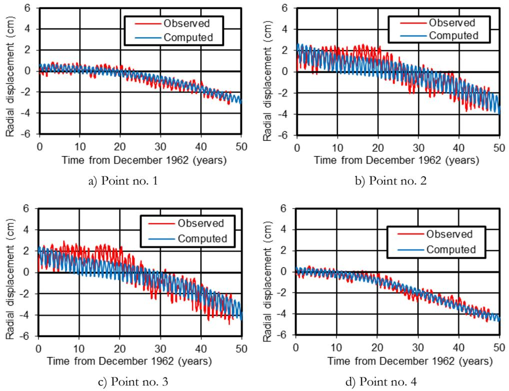
FIGURE 7: Comparison of recorded and computed displacements
