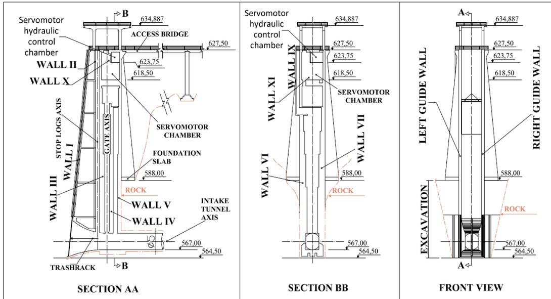
Figure 2: Jaguari HPP water intake showing front view and sections.
