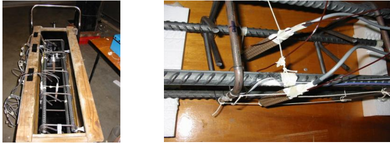
Figure 1- Reinforcement configuration, and close up showing embedded concrete strain gauges
