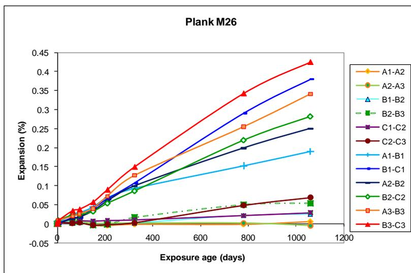
Figure 9- Expansion measurements on planks under outdoor exposure conditions. Locations for A1-A2, A2-A3, B1-B2, B2-B3, C1-C2, C2-C3 are along the planks, whereas A1-B1, B1-C1, A2-B2, B2-C2, A3-B3 and B3-C3 are in the transverse direction, and perpendicular to the existing parallel cracks.
