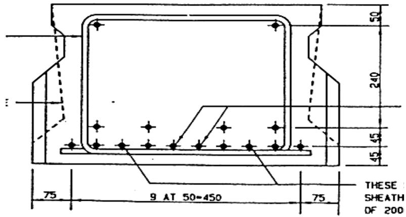
Figure 1- Details of steel reinforcement and prestressing cables in the planks
