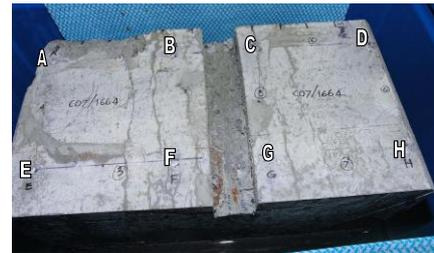
Figure 8- Expansion measured on the surface of sawn Block M26 in the transverse directions A-B, C-D, E-F and G-H, as well as longitudinally in the direction of the prestress D-H, C-G, B-F and A-E
