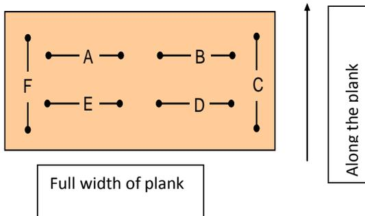
Figure 4- Measurement grid on Blocks cut from the planks (300 x 600 x 380 mm) for expansion measurement at 38°C, 100% RH, in transverse (A, B, D, E) and longitudinal (C, F) directions
