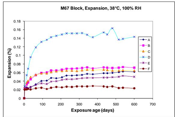
Figure 7- Expansion measured on the surface of sawn Blocks M12 and M67 in the transverse directions A, B,D and E, as well as longitudinally in the direction of the prestress (C and F)
