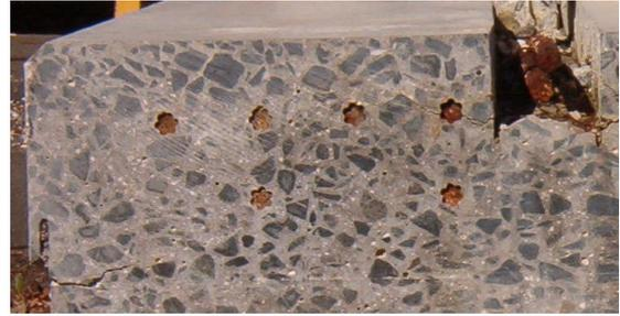
Figure 10- Left: Plank M26 after testing. The expansion measurements grid is on the far left. Right: retraction of prestressing cables (prestress loss) over the period of testing
