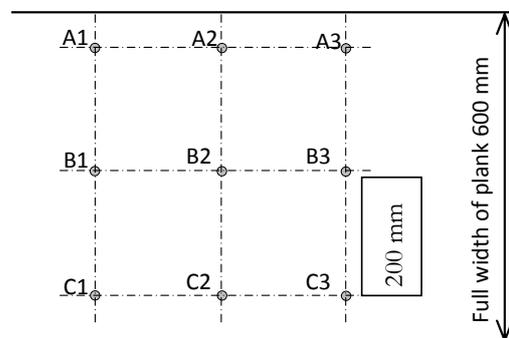
Figure 5- Square grid of expansion measurement points on plank surfaces
