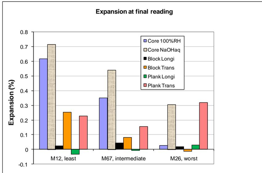
Figure 11- Comparison of expansion measured on planks and different specimens at the end of the testing periods for the test concerned
