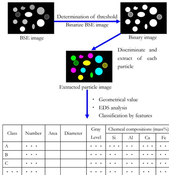
FIGURE 3: Flow diagram of feature analysis
