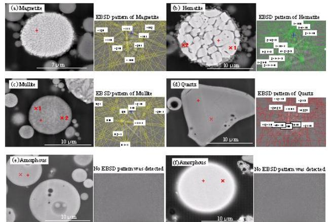
FIGURE 5: BSE images and EBSD patterns of FA particles (+: EBSD, numbers are face index, x: EDS)
