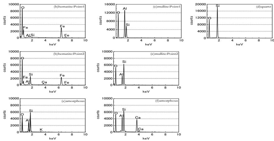
FIGURE 6: EDS spectrums of FA particles (analyzed points are indicated in Figure 5)
