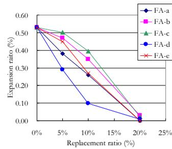
FIGURE 2: FA replacement ratio and 14 d expansion
