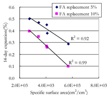
FIGURE 8: Estimated specific surface area of mullite-rich particles and 14-day expansion
