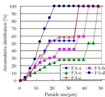
FIGURE 7: Estimated particle size distribution of mullite-rich particles
