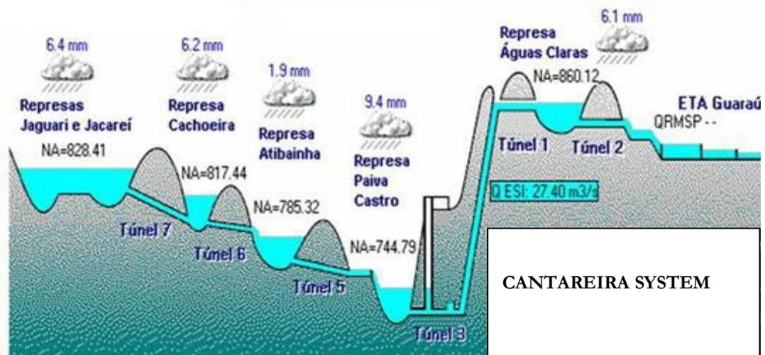
Figure 1- Scheme showing dams and tunnels of the Cantareira System that supplies water to Sao Paulo Metropolitan Region (not on scale).
