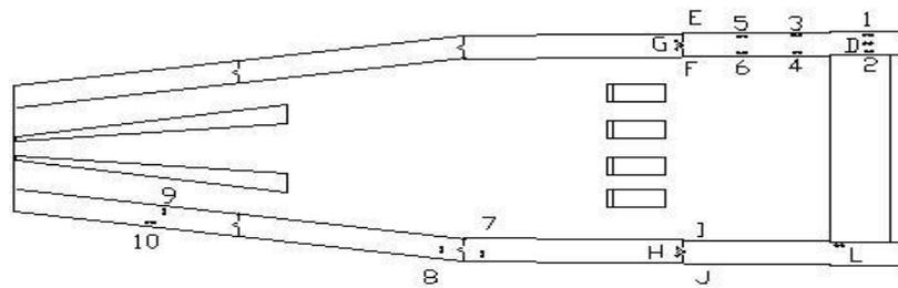
Figure 3 - Plan showing schematic location of pins at the dissipation basin walls of Paiva Castro dam (not on scale).
