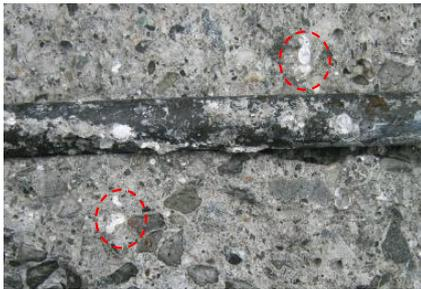
Figure 12: White deposits around steel in specimen. (SC40)
