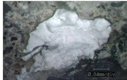
Figure 13: White deposits observed by microscope.
