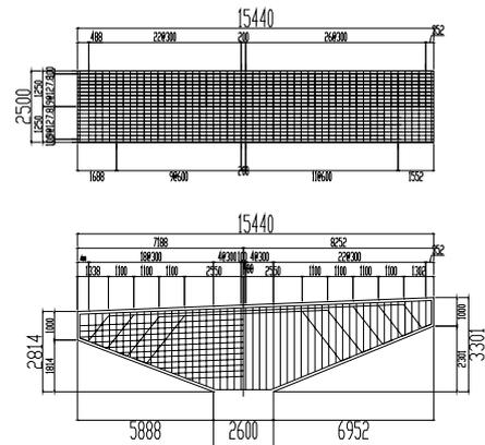
FIGURE 2: Structural drawings of Pier II
