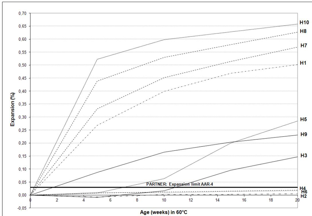
FIGURE 2: RILEM AAR-4 – Expansion results after 20 weeks of exposure in 60°C.
