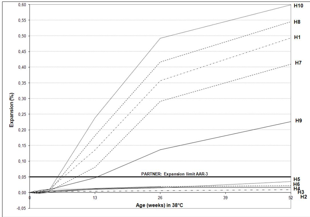
FIGURE 1: RILEM AAR-3 – Expansion results after 52 weeks of exposure in 38°C.
