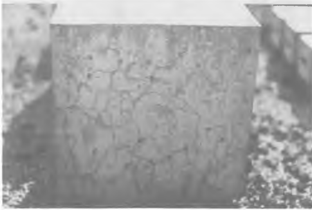
FIGURE 8 VDZ "Large cube" test for assessing reactivity of cement and aggregate combinations
