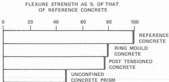
Figure 4. Flexure strength of concrete samples plotted as a percentage of that of reference concrete
