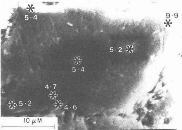
Figure 6. SEM micrograph of dolomitic rhomb in polished slab of reacted dolomitic limestone aggregate. (The location of the areas analysed is shown by \*. The number beside the \* gives the Ca/Mg count ratio)
