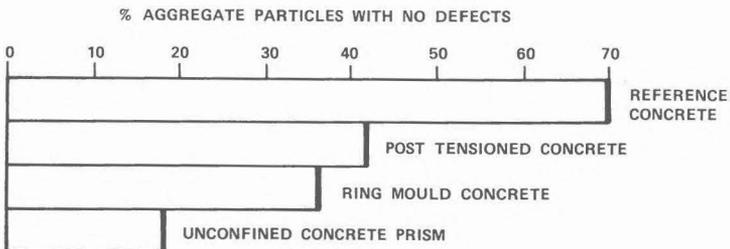
Figure 3b. Percentage of aggregate particles (in four concrete samples) with no defects, i.e., without reaction rims or cracks
