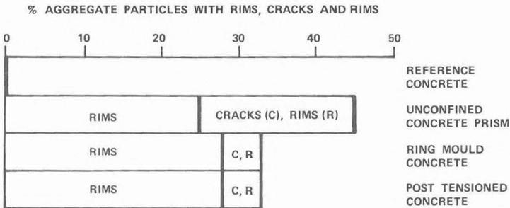
Figure 3a. Percentage of coarse aggregate particles with reaction rims or a combination of cracks and rims
