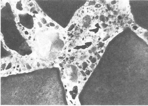
Figure 5. Dark reaction rims around particles of reactive dolomitic limestone aggregate in concrete
