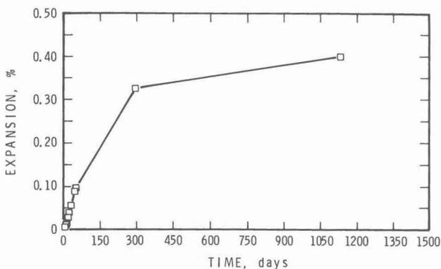
Figure 1. Expansion of unconfined concrete prism made with reactive alkali-carbonate aggregate and high alkali cement
