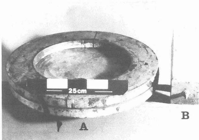
Figure 2. A -- Ring mould made from 2.5-cm thick steel plate
