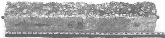
(A) Prism Cut From the Pre-Cast Panel (40 x 40 x 285 mm)
