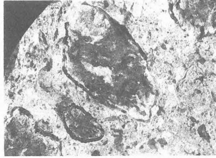
Fig 2 ASR in Granitic rocks
