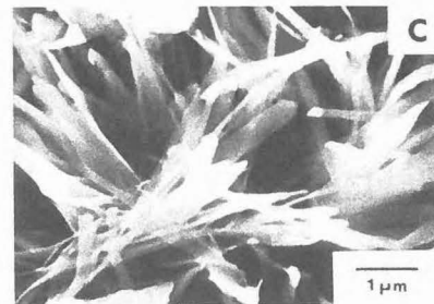
Fig.7. Various crystal habits from white reaction rim on metadolerite aggregates: (a) mixture of amorphous and crystalline material, (b) crystals not well formed, and (c) highly crystalline AAR products. All forms contain Si, Ca, Na, K.
