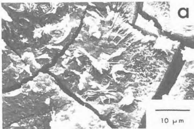
Fig. 4. Gel-filled cracks around reacted aggregate and in the mortar. Crossed polarized light.
