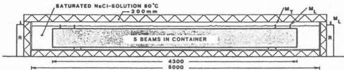
Figure 2. Storage tank for concrete beams with saturated NaCl solution at 50°C.  $M_L$  are measuring points for longitudinal expansion;  $M_T$  are measuring points for transverse expansion.
