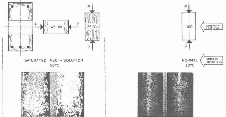
Figure 6. P is the direction of compression. The crack system in the beams is moving inwards with increasing storage time.
