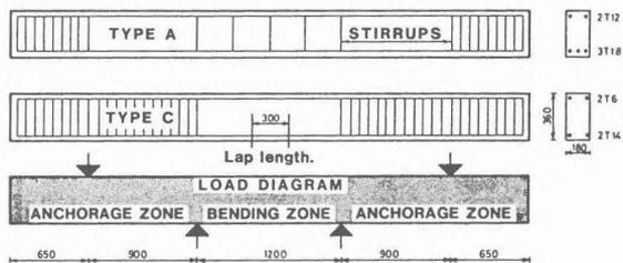
Figure 1. Test beams, geometry, reinforcement, and load diagram
