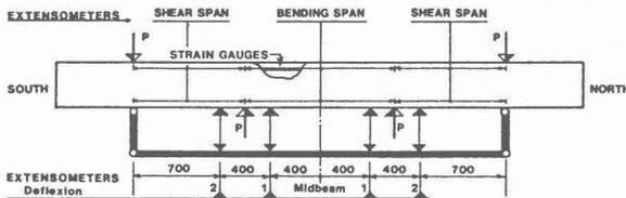
Figure 5. Principle of the shear test set-up.
