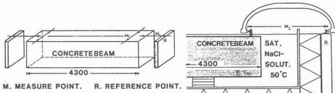
Figure 3. The R measuring points are placed on a steel profile, and each of them is fixed to the concrete floor with four 18 mm steel expansion bolts.
