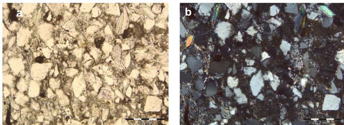
Figure 3.3: Cross sections of the coarse aggregate recognised as a sandstone (thin section, scale bar = 0.2 mm, PPL (a) and XPL (b))
