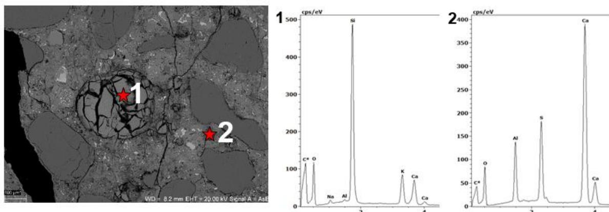
Figure 3.4: Scanning electron micrograph of the air void filled with ASR gel (1) and ettringite (2)
