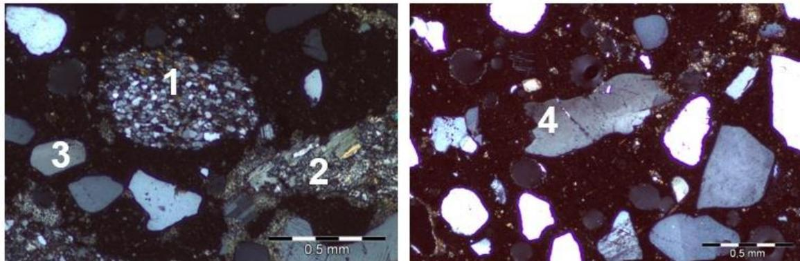
Figure 3.1: Cross sections of the fine aggregates (thin section, XPL, scale bar = 0.2 mm), 1 - microcrystalline quartz, 2 - micro- and cryptocrystalline quartz, 3 - monomineral quartz, 4 - strained quartz
