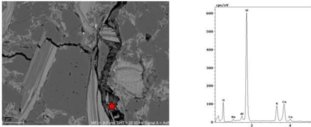
Figure 3.5: Scanning electron micrograph of the cracked aggregate grain filled with Si-Ca-K-Na gel
