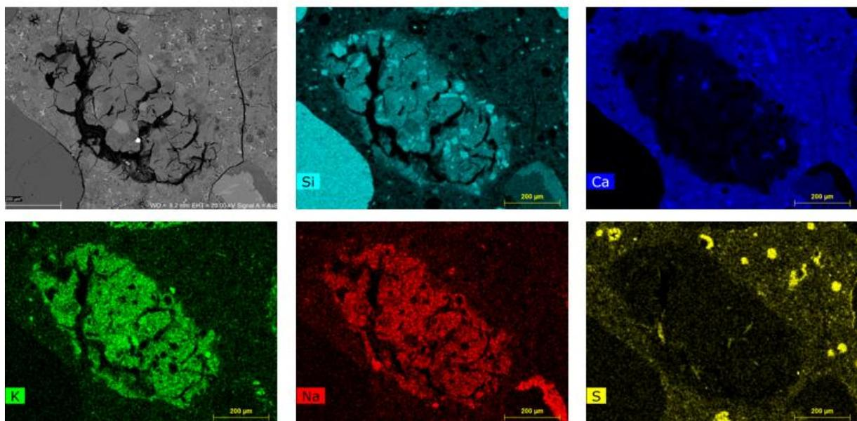
Figure 3.9: EDS mapping of the reacted aggregate grain (almost completely converted into a ASR gel)
