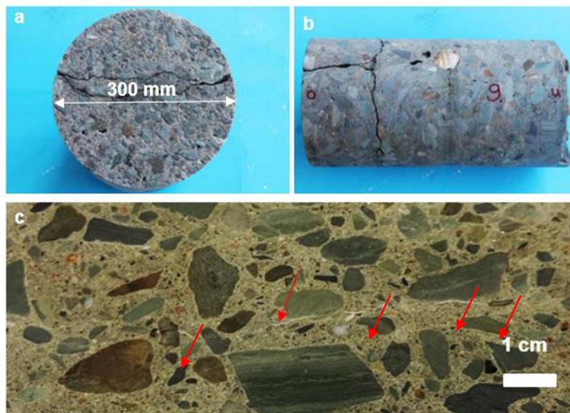
Figure 2.1: a, b) Photographs of a core from concrete pavement, c) lapped surface of Core 9 from concrete expressway showing a crack radiating from a rimmed, dark schist particle into adjacent paste. The crack is filled with white gel
