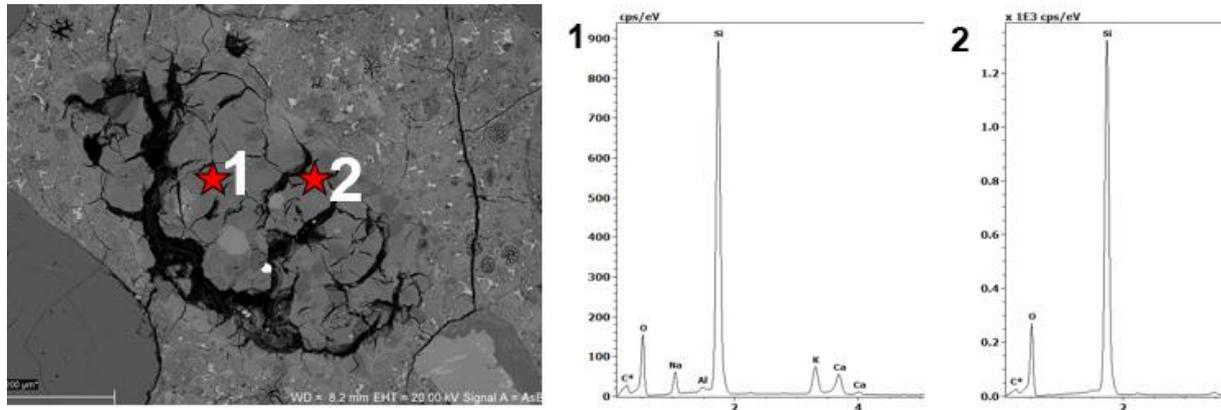
Figure 3.8: Scanning electron micrograph of the reacted aggregate grain almost completely converted into Si-Ca-K-Na gel, with remnants of quartz
