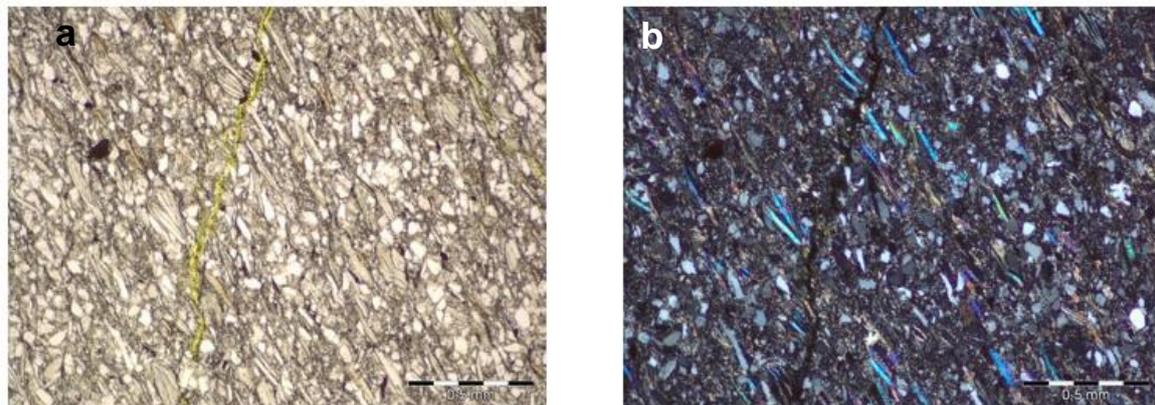
Figure 3.2: Cross sections of the coarse aggregate grain recognised as a schist (thin section, scale bar = 0.5 mm, PPL (a) and XPL (b))
