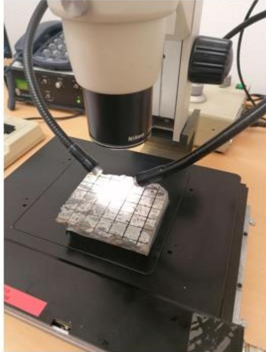
Figure 2.2: Stereoscopic microscope with analyzed polished concrete section 10 x 10 cm with grid (1,5 x 1,5 cm) on an automatic table
