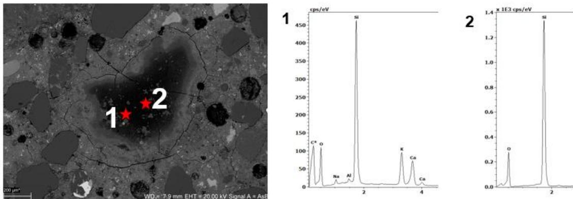
Figure 3.7: Scanning electron micrograph of the reacted aggregate grain almost completely converted into Si-Ca-K-Na gel, with remnants of quartz
