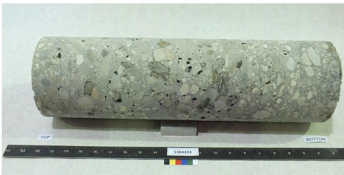
Figure 3.1: Photograph of air dried core from Mix 1, showing wet rims around coarse aggregate indicative of ASR.
