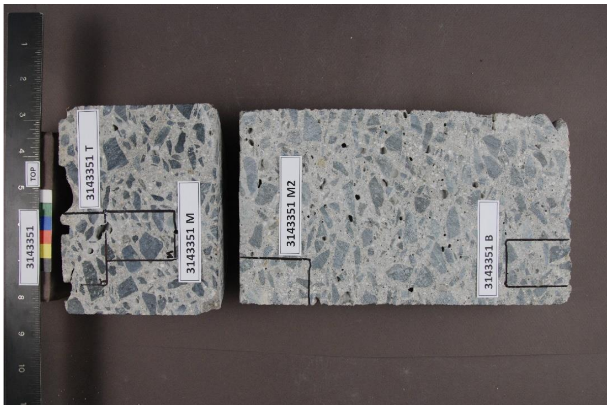
Figure 2.3: Photograph of cross-sectioned core showing locations of thin section preparation outlined in black.
