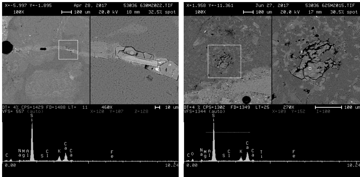
Figure 3.4: Backscattered electron (BSE) images with EDS spectra of ASR gel within pockets in Coarse Aggregate 2.
