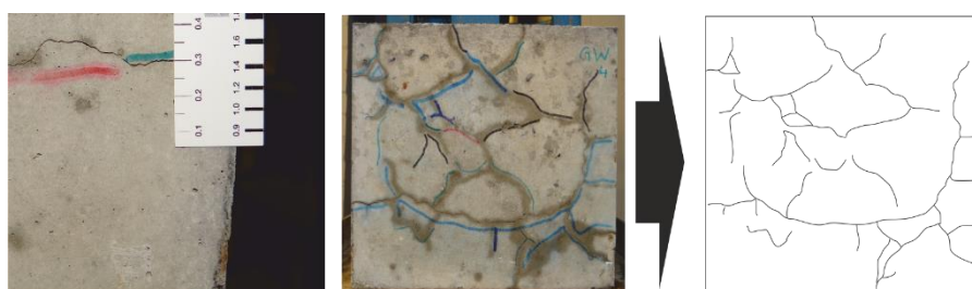
Figure 2.2: Example of the documentation of the cubes during the ASR-provoking storage in the fog-chamber
