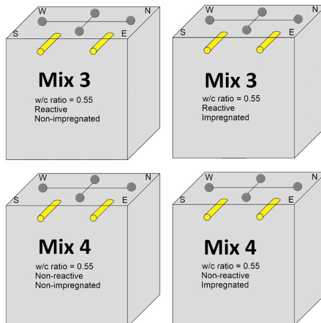
Figure 2.4: The concrete cubes for mix 3 and 4 with a w/c-ratio at 0.55 equipped with measurement studs (the grey dots) at the top, the south/west side and west/north side of the cubes, where southwest side and northwest side are not shown.
