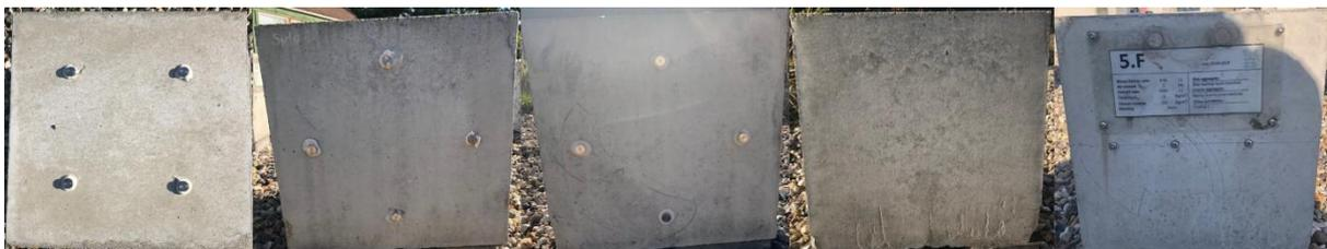
Figure 4.4: Crackmapping picture of concrete cube – mix 3 – impregnated - 998 days after casting.
