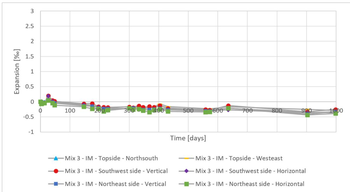
Figure 3.4: The expansion measurements for impregnated cube with mix 3 (IM = impregnated).
