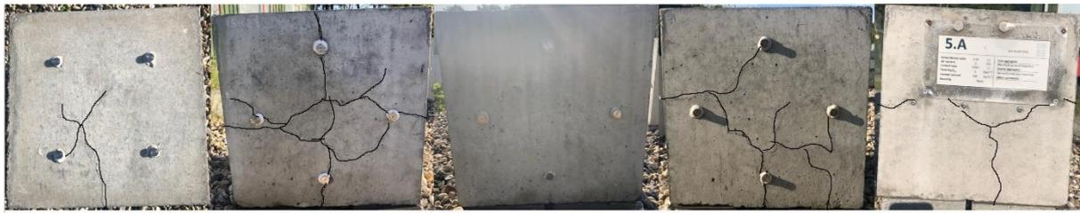
Figure 4.1: Crackmapping picture of concrete cube - mix 1 - non-impregnated - 1008 days after casting.
