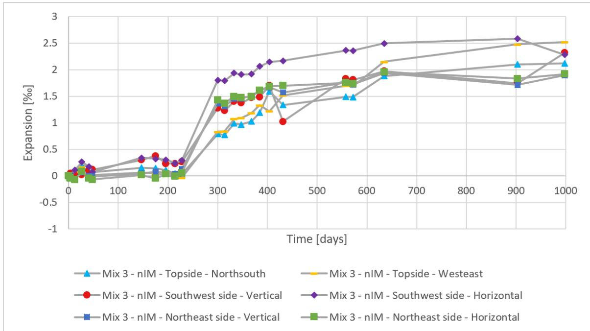
Figure 3.3: The expansion measurements for non-impregnated cube with mix 3 (nIM = non-impregnated).
