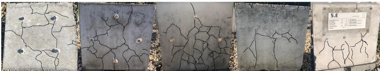
Figure 4.3: Crackmapping picture of concrete cube – mix 3 – non-impregnated - 998 days after casting.
