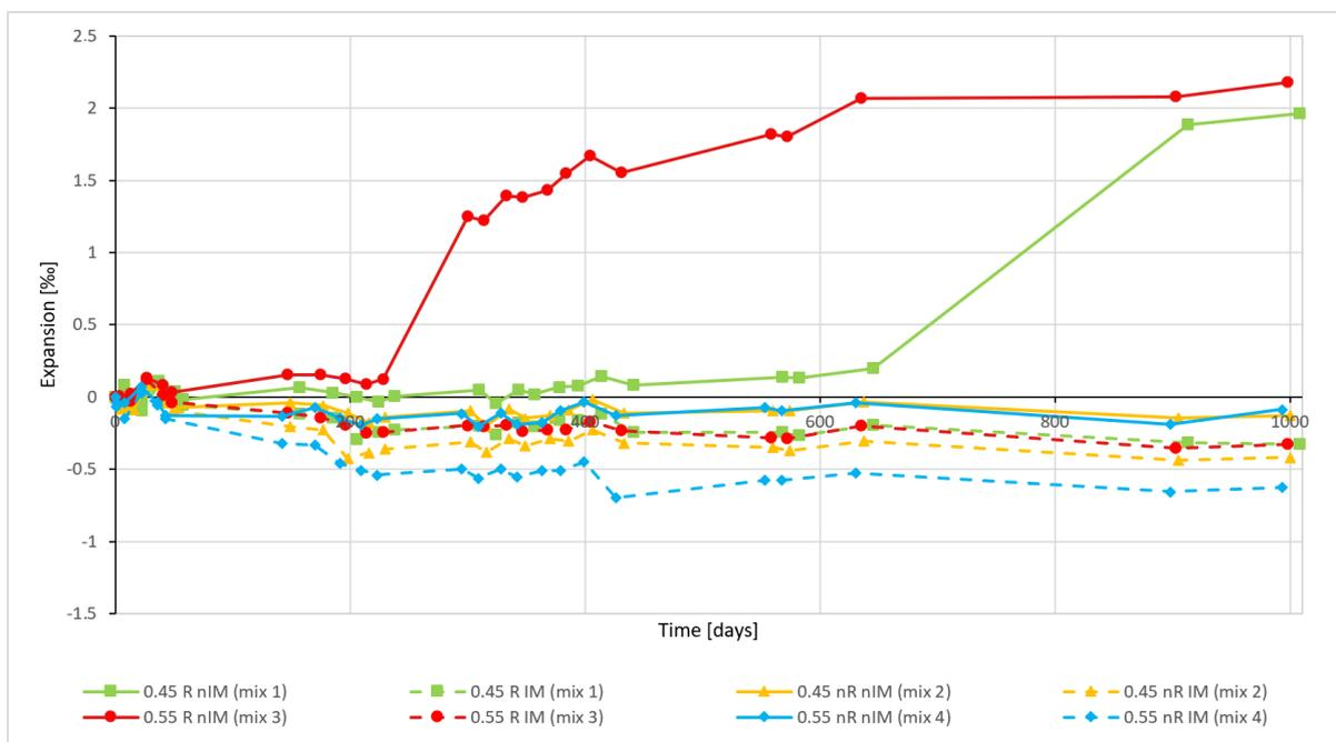
Figure 3.2: The average expansion results for the 8 cubes (R = reactive, nR = non-reactive, IM = impregnated and nIM = non-impregnated).
