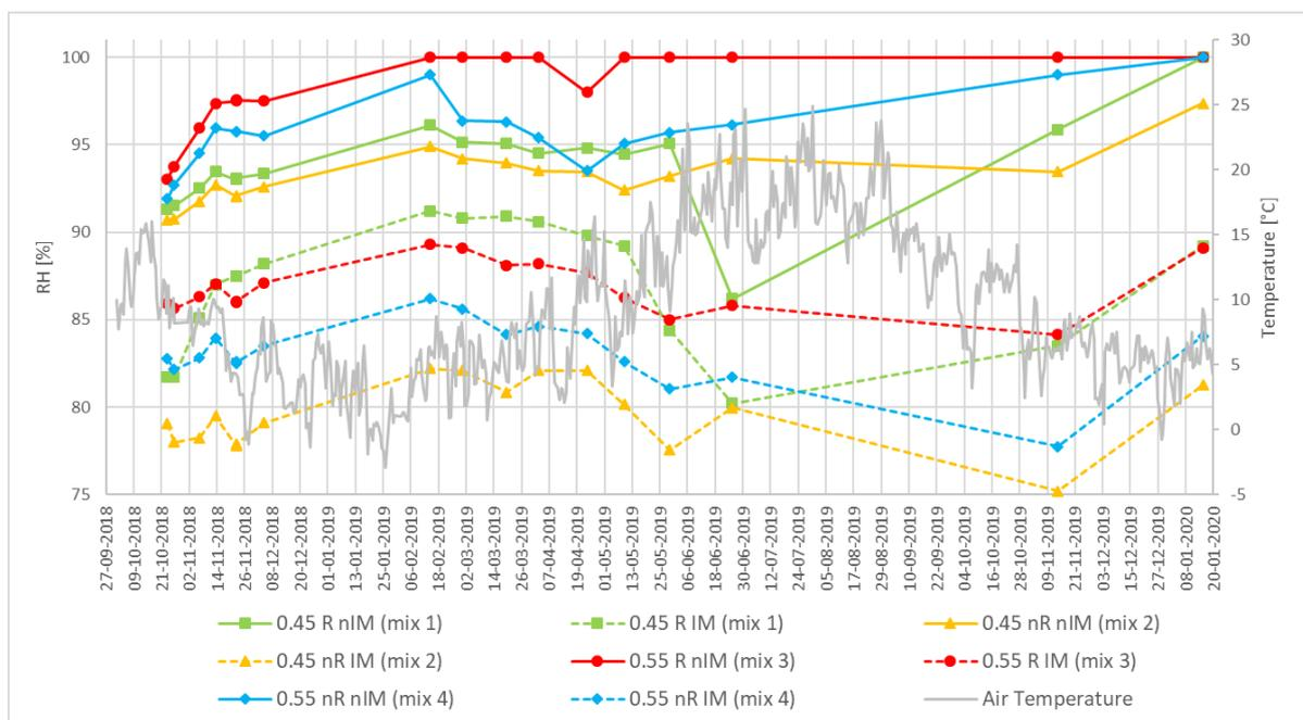
Figure 3.1: The average relative humidity results for the 8 cubes (R = reactive, nR = non-reactive, IM = impregnated and nIM = non-impregnated) and the outdoor air temperature.
