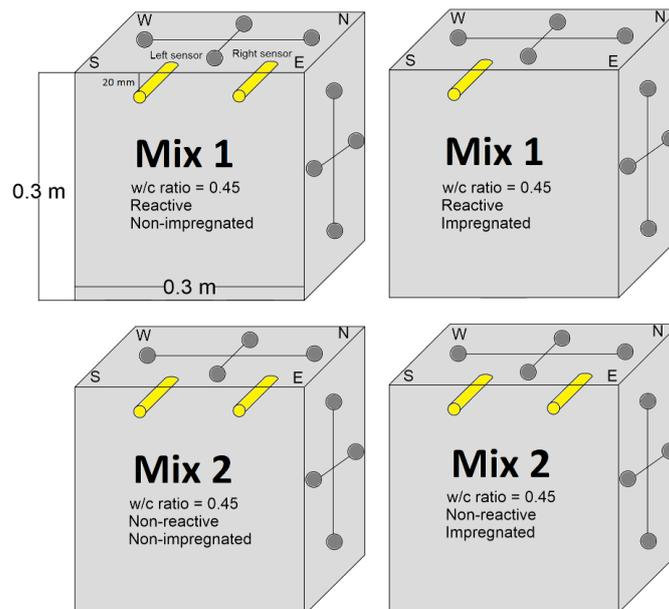
Figure 2.3: The concrete cubes for mix 1 and 2 with a w/c-ratio at 0.45 equipped with measurement studs (the grey dots) at all sides of the cubes except of the south/east side and the bottom, where southwest side and northwest side are not shown.
