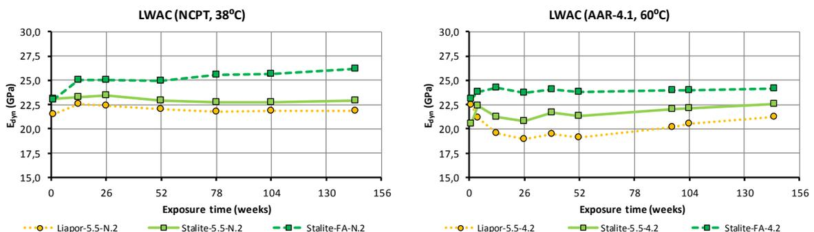
Figure 3.3: Development of Young's Dynamic modulus of elasticity ( $E_{dyn}$ ) of prisms when exposed to NCPT and AAR-4.1 conditions, respectively.
