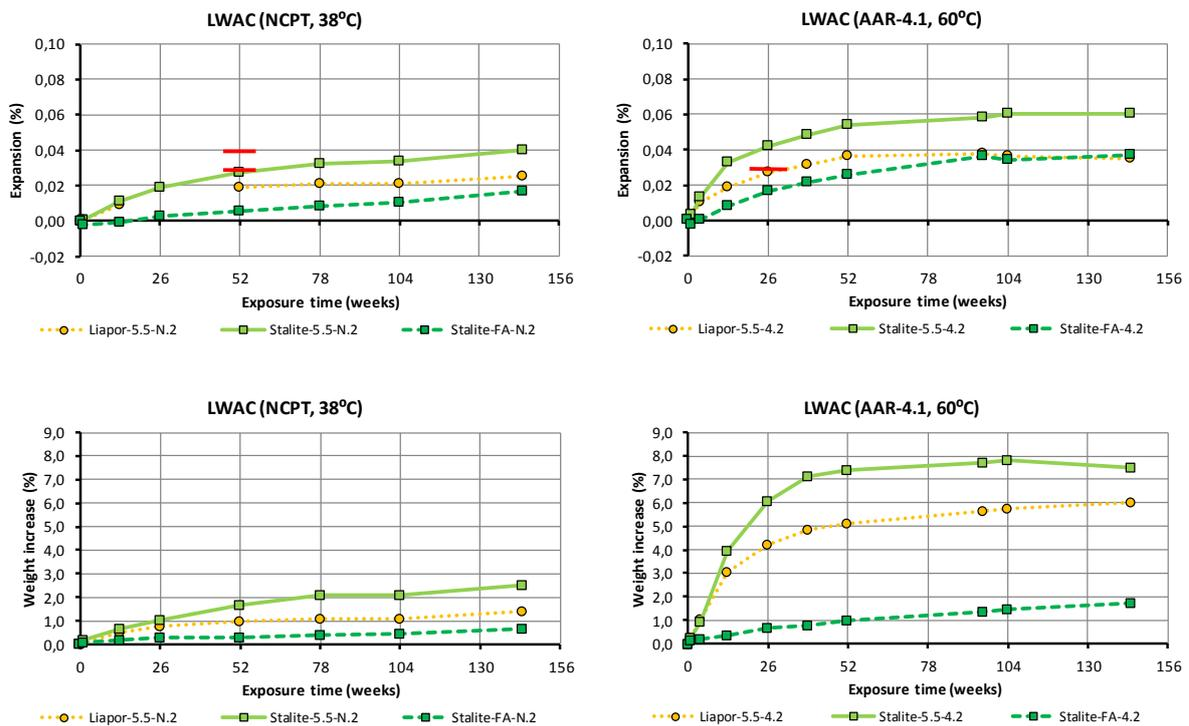
Figure 3.2: Expansion (upper) and weight increase (lower) of prisms testing according to the NCPT and AAR-4.1. Red lines indicate the respective recommended acceptance limits.
