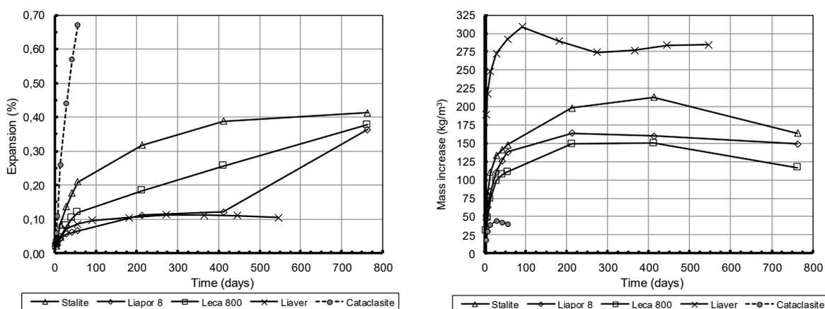
Figure 3.1: Expansion (left) and mass increase (right) of mortar bars submerged in 1M NaOH at 80°C [5]. The four LWAs are compared with the normal density alkali-reactive cataclasite aggregate [1]
