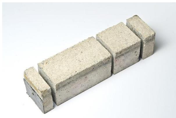
Figure 2.3: Cut prism after FIB climate test method for testing compressive strength, modulus of elasticity, creep and shrinkage (from [20])
