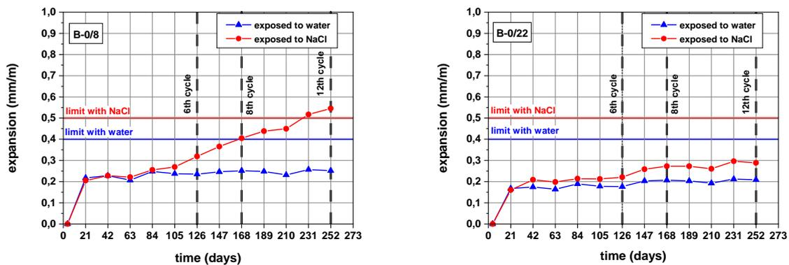
Figure 3.2: Results of expansion measurements, concrete compositions B-0/8 and B-0/22
