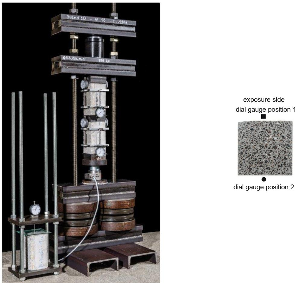
Figure 2.4: Example of the test rig for creep and shrinkage (from [14]) and an example for the positions of the dial gauges
