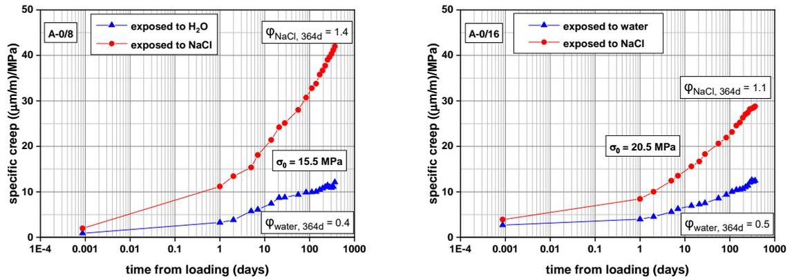
Figure 3.3: Specific creep, concrete compositions A-0/8 and A-0/16
