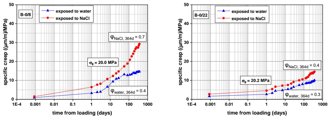
Figure 3.4: Specific creep, concrete compositions B-0/8 and B-0/22
