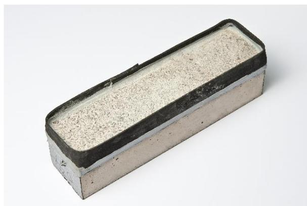
Figure 2.1: Prepared prism for the FIB climate test method (from [20])
