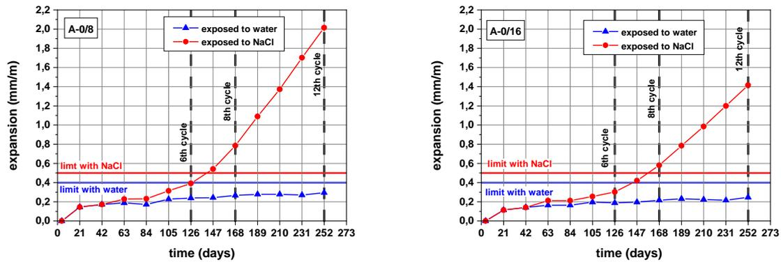
Figure 3.1: Results of expansion measurements, concrete compositions A-0/8 and A-0/16
