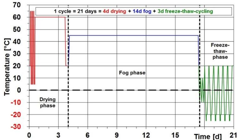
Figure 2.2: Temperature scheme for one cycle of the FIB climate test method [21]
