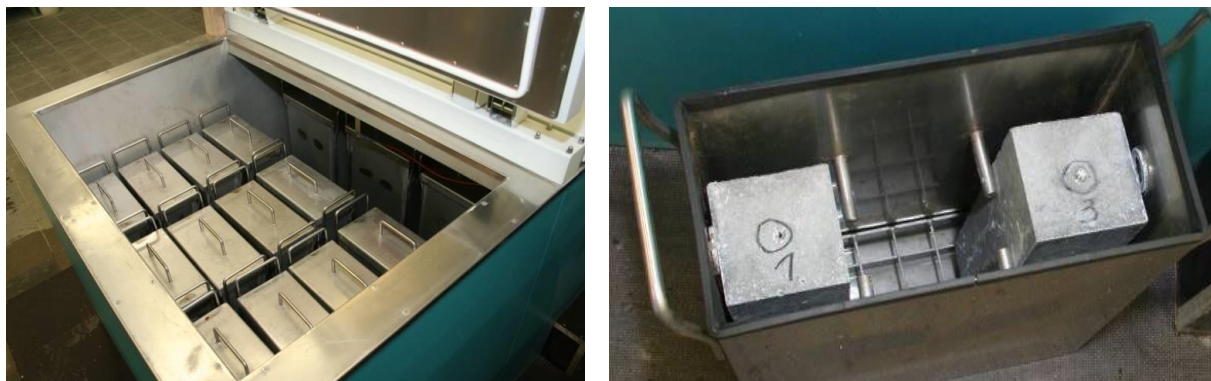
Figure 3.2: Typical containers for RILEM AAR-11 that have proven to be suitable for storage; three specimens per small container; the small containers are stored at 60°C inside a humid reactor.
