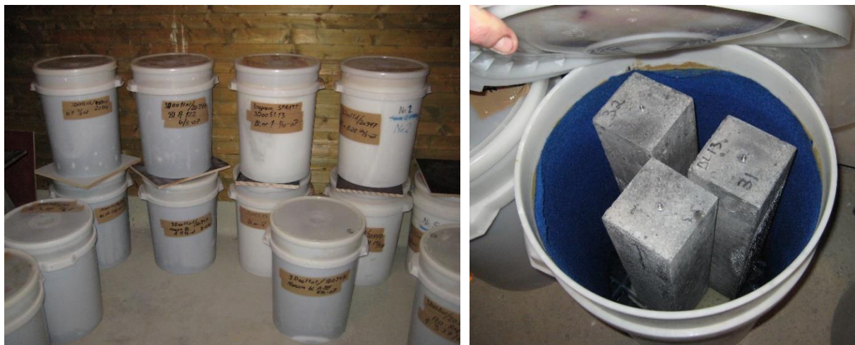
Figure 3.1: Typical containers for RILEM AAR-10 that have proven to be adequate for storage; three specimens per container; the containers are stored in a 38°C dry room.
