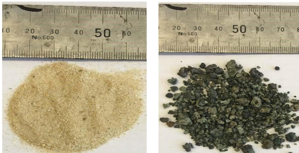
Figure 2.1: Photographs of fine aggregates: sand (left) and FNS (right) Table
